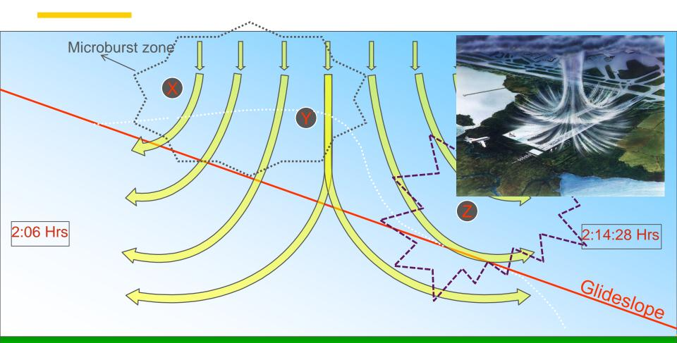
The aircraft encounters point X, where it enters the microburst zone, and a headwind causes it to rise above the normal glideslope. At the center of the microburst, point Y, there is a downdraft causing the aircraft to sink. The aircraft now enters the most dangerous zone, point Z, where a sudden tailwind causes the aircraft to lose airspeed and potentially crash. F-7-14-54 (AF477)
