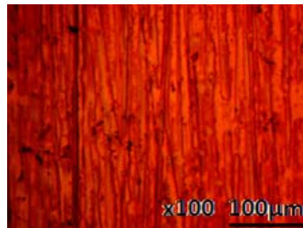
Fig. 8. Optical microscopy image of untested S41003 sample
