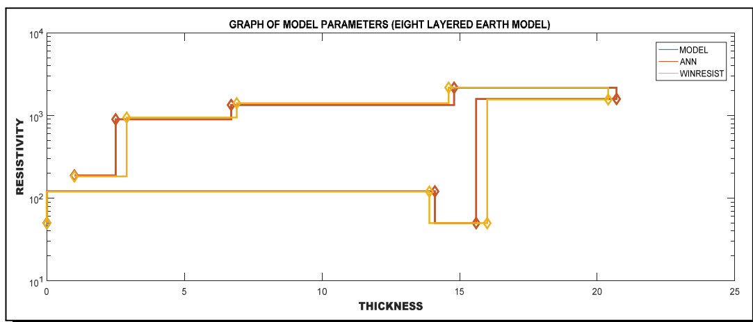
Figure 9. ANN responses compared with synthetic model parameter for eight layered earth model
