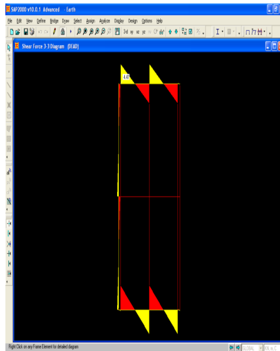
Fig. 6 Shear force diagram of earth plastered typha strawbale wall
