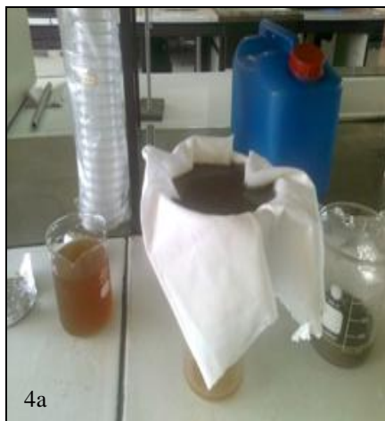
FIG. 4a: FILTRATION SETUP OF OBTAINING GLUCOSE SYRUP FROM THE WORT
