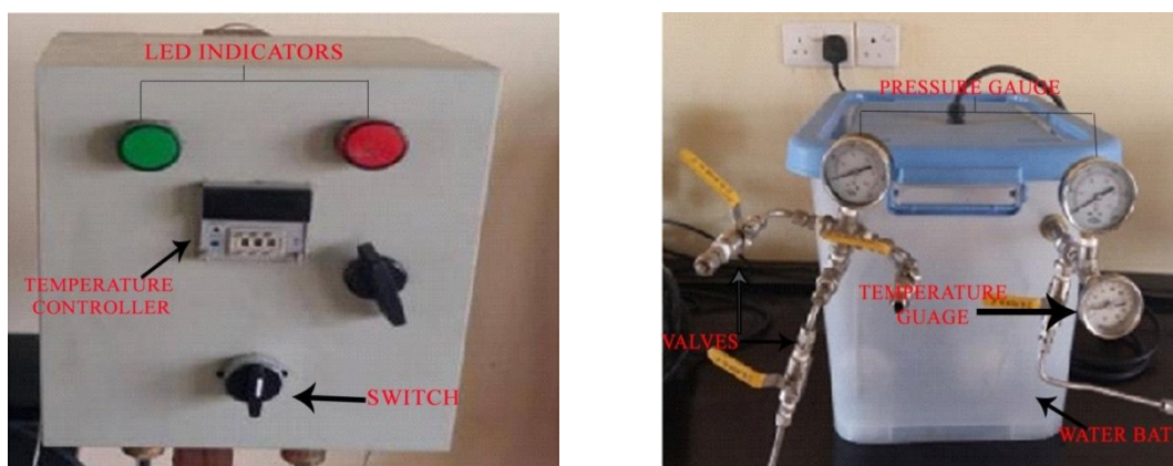
Fig. 2. Fabricated sorption isotherm equipment for Nigerian coal
