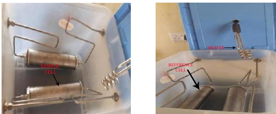
Fig. 1. Fabricated reference and sample cell
