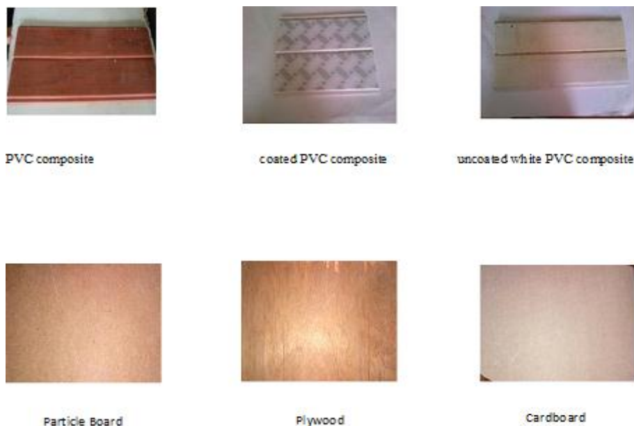
Plate: Samples of PVC and natural Ceiling Materials
