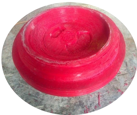
Figure 6. FDM-printed PLA-pattern for sand casting
