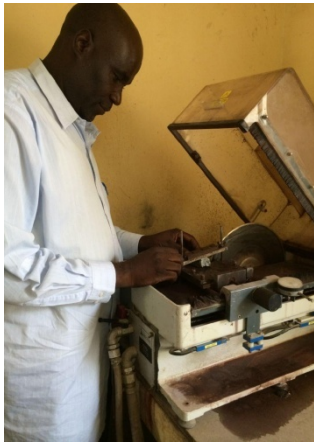
Figure 1. Alogitech GTS 1 Thin Section Cut Off Saw
