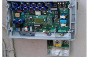
**Figure 2: Solar Inverter**
