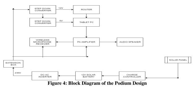
The block diagram above (figure 4) shows the working principle of the podium. The solar panel harnesses light energy from the sun in other to generate electricity. The solar charge controller in the podium makes sure maximum power is transferred to the solar battery. The inverter is connected to the battery to allow the AC devices in the podium to work with the 12v battery.
