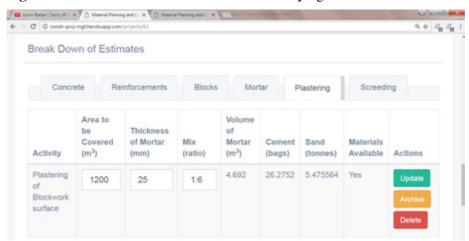
Figure 7 Screen shot of estimate in plastering blockworks
