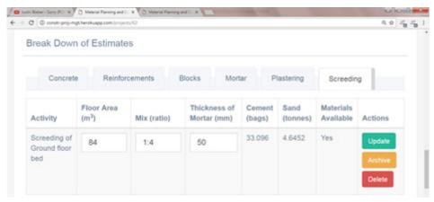
Figure 8 Screen shot of estimate in screeding concrete floor surfaces
