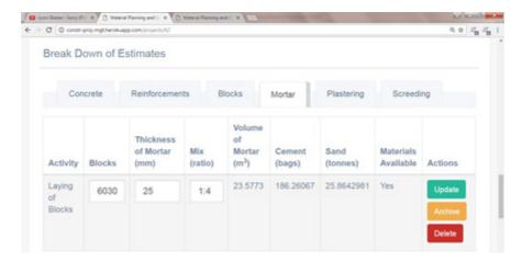
Figure 6 Screen shot of estimates for mortar in laying of sandcrete blockwalls
