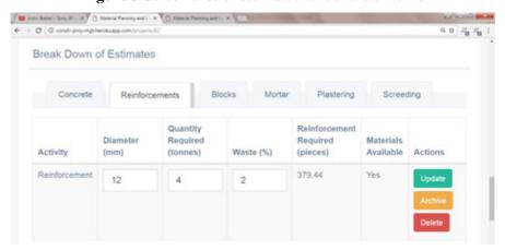
Figure 4 Screen shot of estimates for steel reinforcement details
