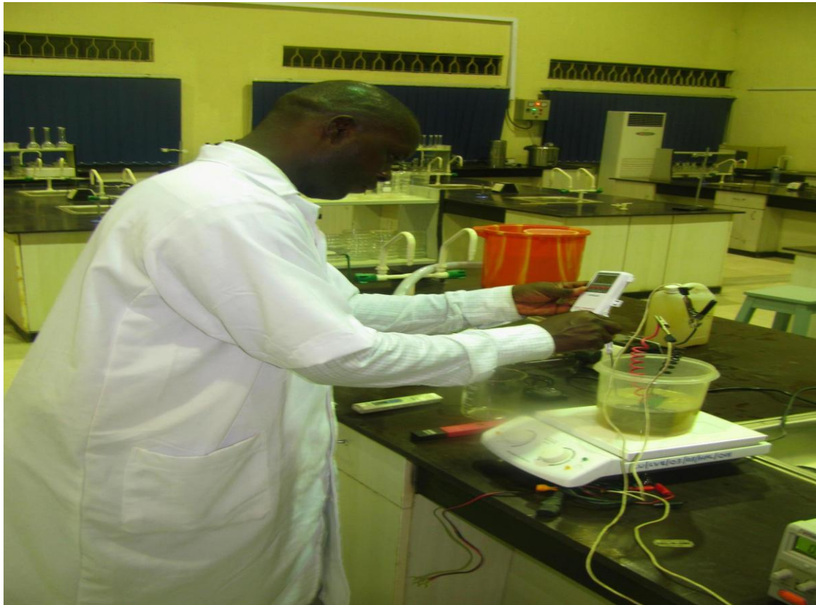
PLATE XIII Measuring water quality parameters from Laboratory Bench- Scale Electro – Fenton Experiment
