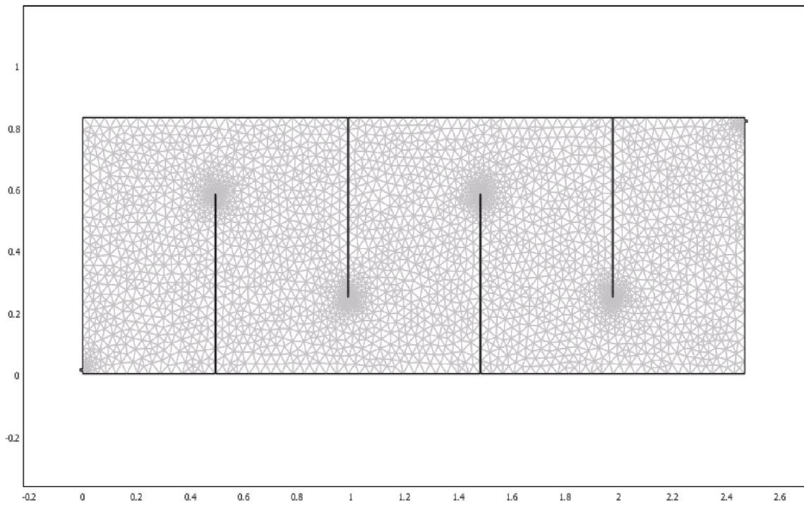
**Figure 3.22** Mesh structure in a 4 baffled 70% Transverse Maturation reactor
