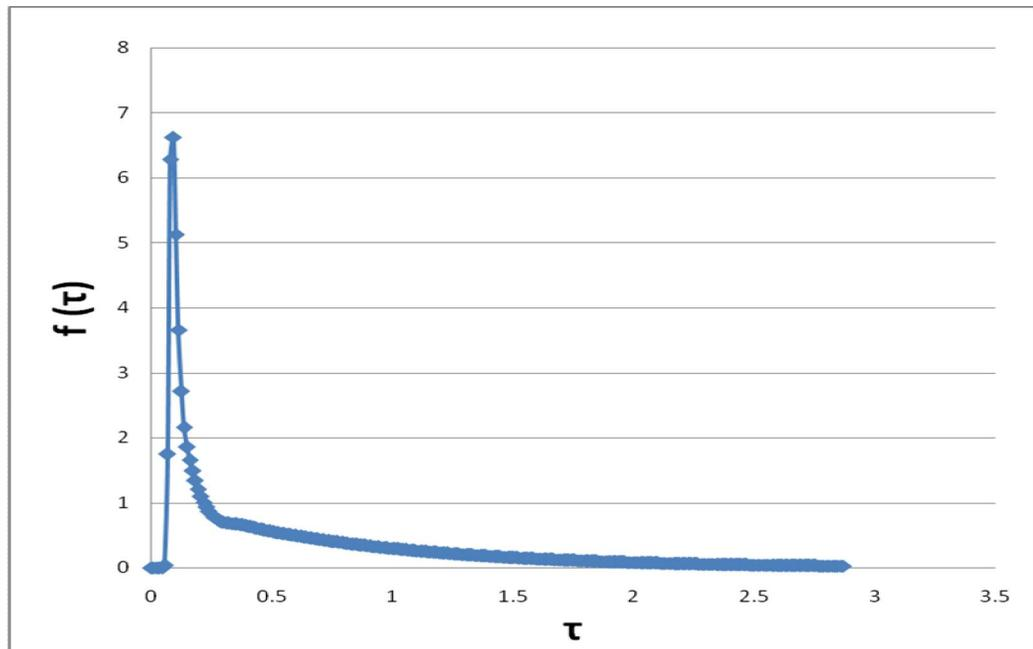
**Figure 4.3** Residence time distribution curve for un baffled facultative reactor
