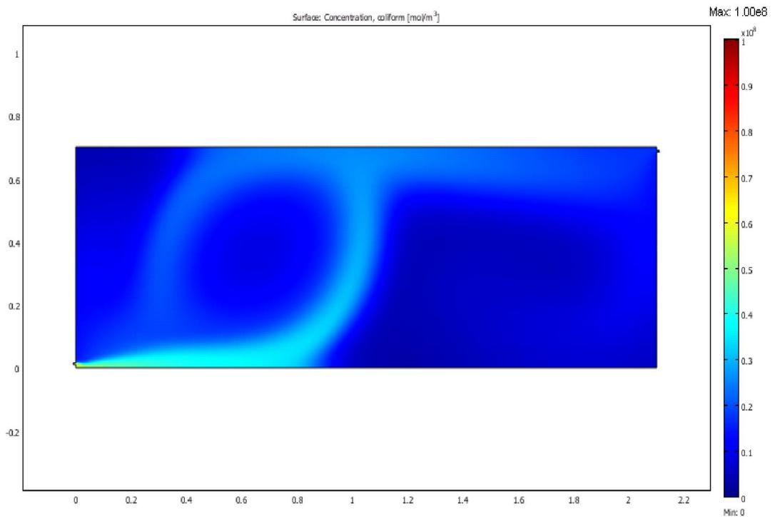
**Figure 4.4** Facultative un baffled reactor coliform inactivation
