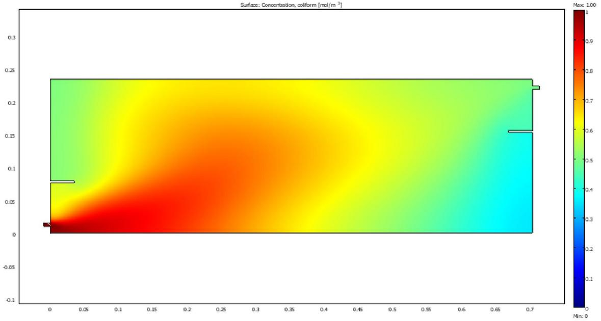
**Figure 4.87** MOGA II sensitivity analysis optimal faecal coliform removal design with least cost for longitudinal baffle arrangement in anaerobic reactor ( $k = 4.562$ )
