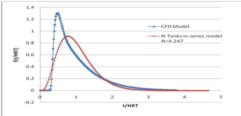
**Figure 4.24** Comparison of residence time density curves in 4-baffles, 70% Pond width Maturation reactor for CFD and N-tanks in series models
