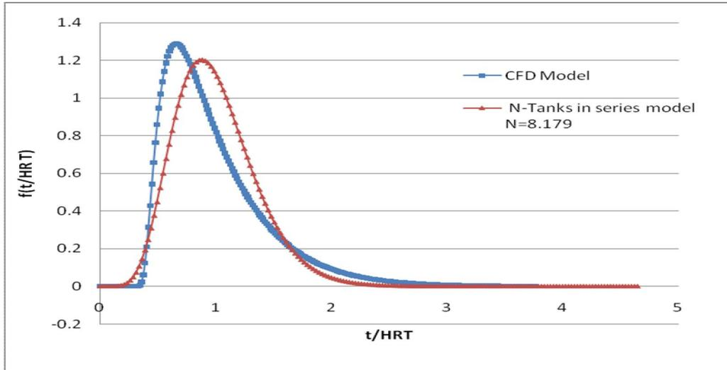
**Figure 4.25** Comparison of residence time density curves in 6-baffles, 70% pond width Maturation reactor for CFD and N-tanks in series models
