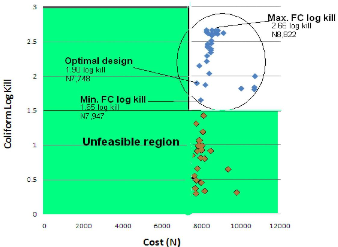
**Figure 4.61** Trade off plot for maturation longitudinal design space.
