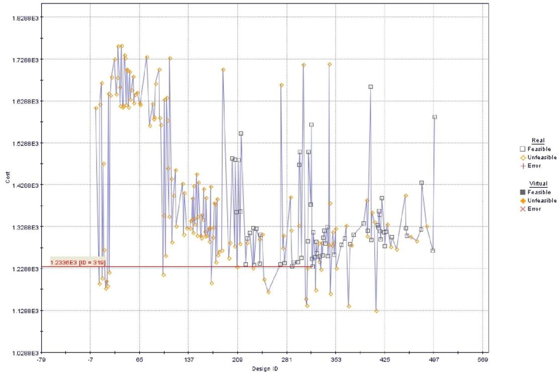
**Figure 4.48** MOGA-II history cost on design for transverse baffle arrangement in anaerobic reactor
