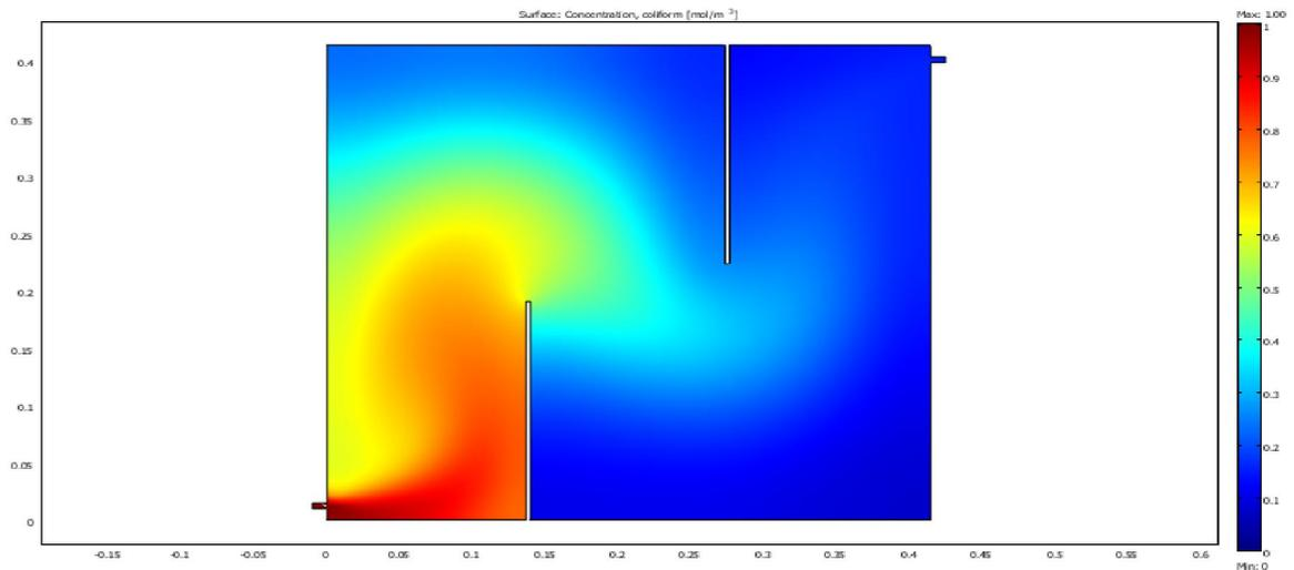
**Figure 4.78** MOGA II sensitivity analysis optimal faecal coliform removal design with least cost for transverse baffle arrangement in anaerobic reactor ( $k = 13.686$ )
