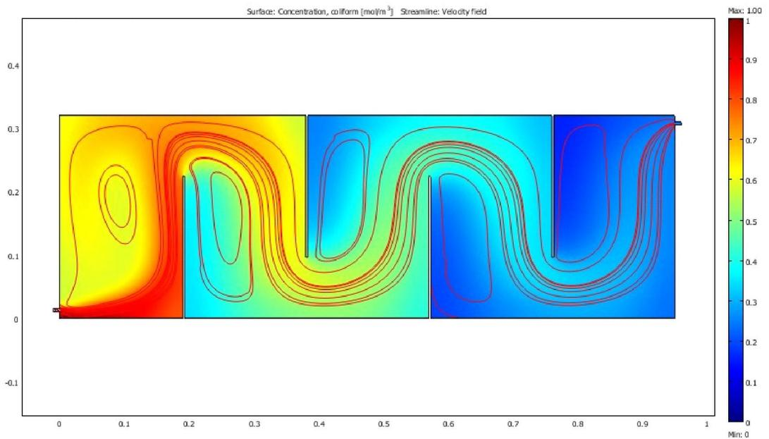
**Figure 4.9** Velocity streamline and coliform inactivation for transverse 4 baffle 70% pond width anaerobic reactor.
