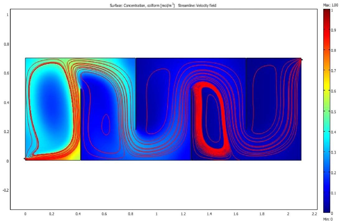
**Figure 4.11** Velocity streamline and coliform inactivation for transverse 4 baffle 70% pond width facultative reactor
