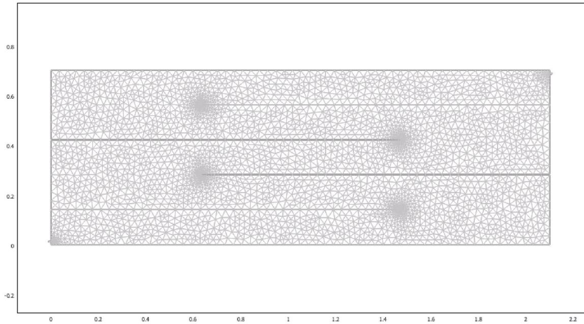
**Figure 3.21** Mesh structure in a 4 baffled 70% Longitudinal Facultative reactor
