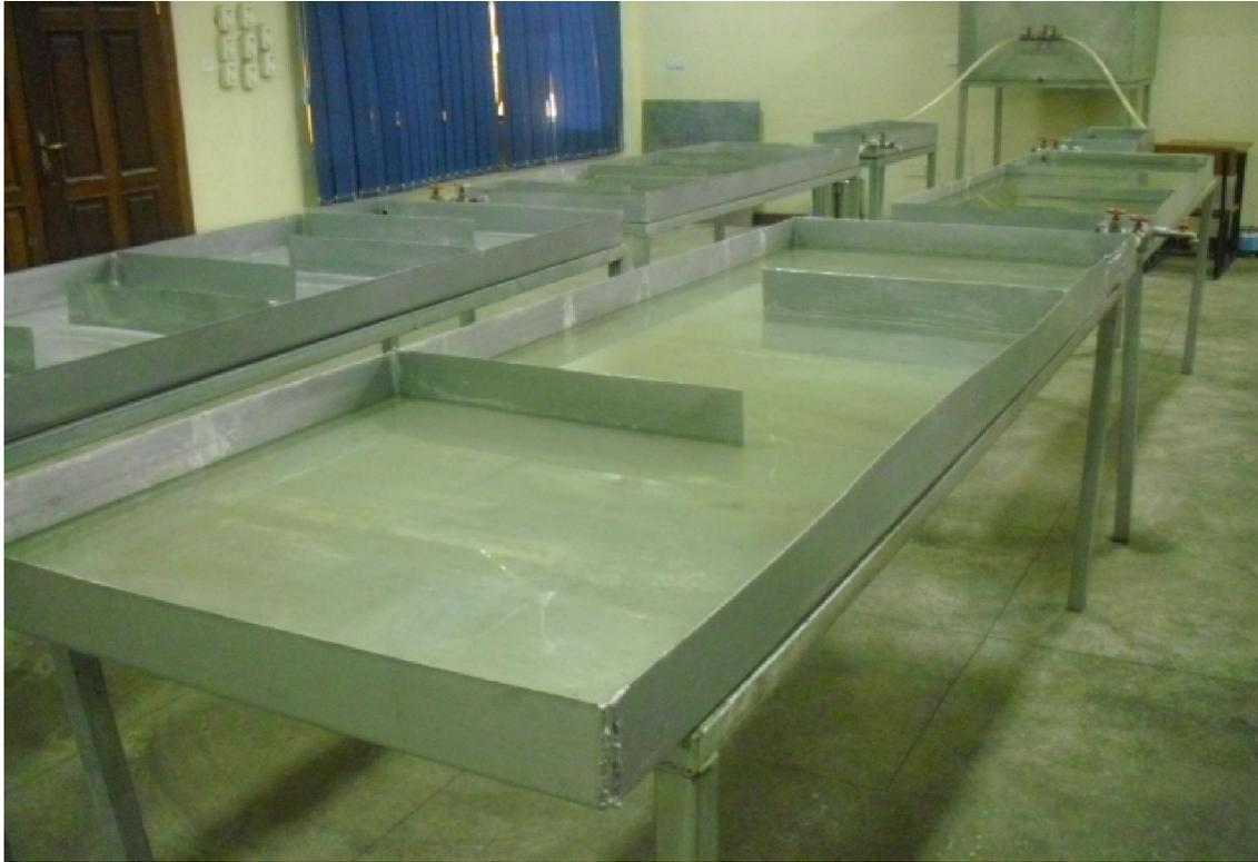
**Plate 3.12** Laboratory-scaled maturation reactors
