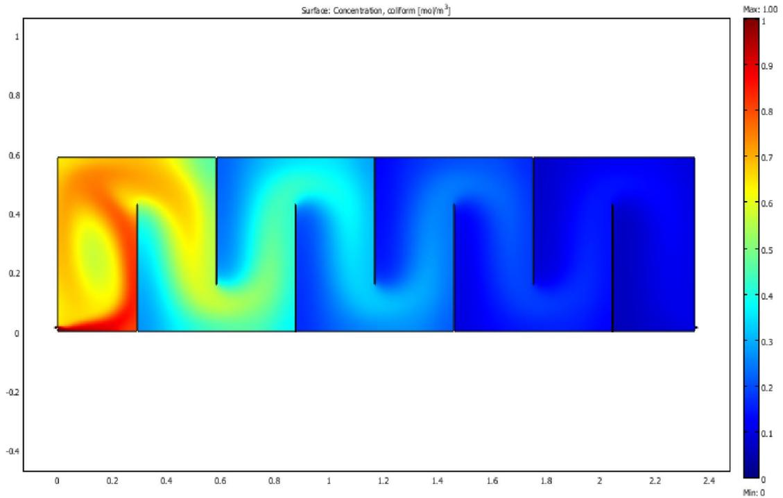
**Figure 4.73** SIMPLEX sensitivity optimal faecal coliform removal design with least cost for transverse baffle arrangement in facultative reactor ( $k = 4.562$ )
