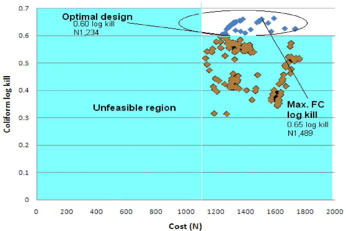
**Figure 4.51** Trade off plot for Anaerobic Transverse design space.
