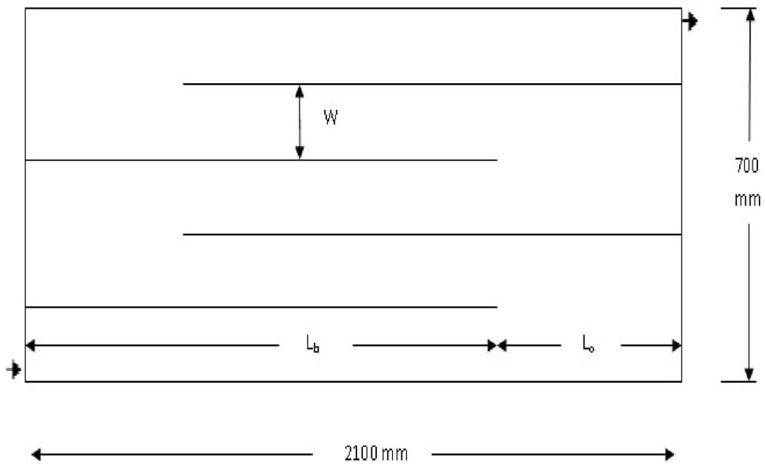
**Figure 3.16** General arrangements of conventional longitudinal baffles of different lengths in the facultative reactor.
