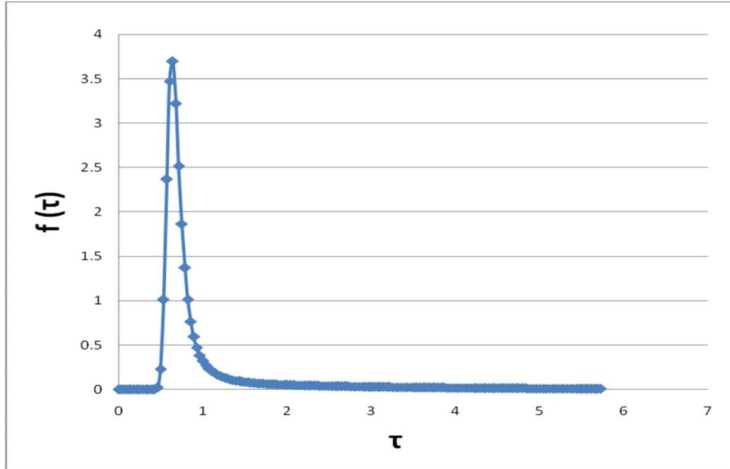
**Figure 4.14** Residence time distribution curve for longitudinal 4-baffle with 70% pond width anaerobic reactor
