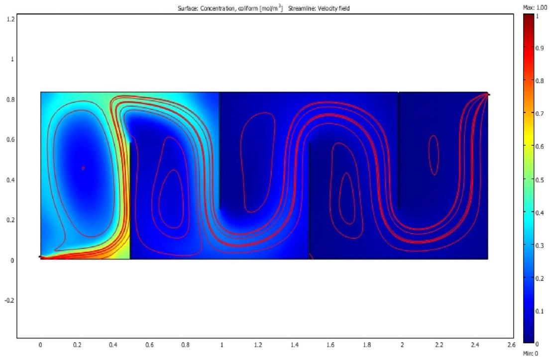
**Figure 4.13** Velocity streamline and coliform inactivation for transverse 4 baffle 70% pond width Maturation reactor
