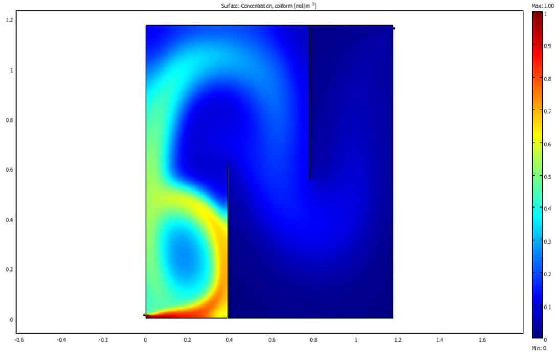
**Figure 4.56** MOGA-II optimal faecal coliform removal design with least cost for even baffle transverse arrangement in facultative reactor
