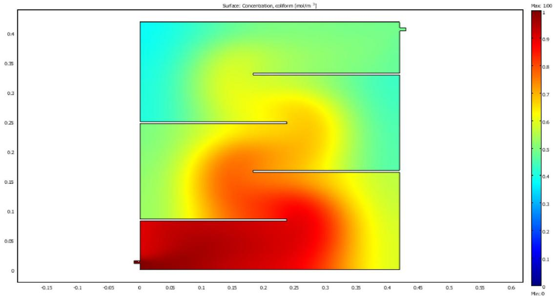
**Figure 4.75** SIMPLEX sensitivity optimal faecal coliform removal design with least cost for longitudinal baffle arrangement in anaerobic reactor ( $k = 4.562$ )
