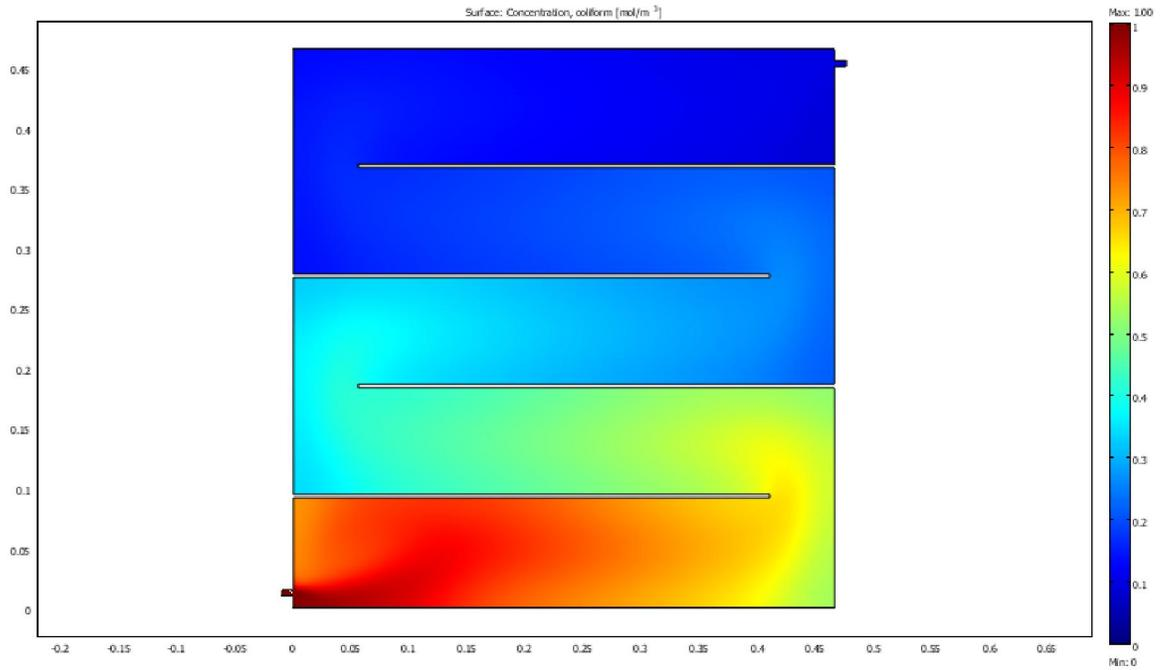
**Figure 4.81** MOGA II sensitivity analysis optimal faecal coliform removal design with least cost for longitudinal baffle arrangement in anaerobic reactor ( $k = 13.686$ )
