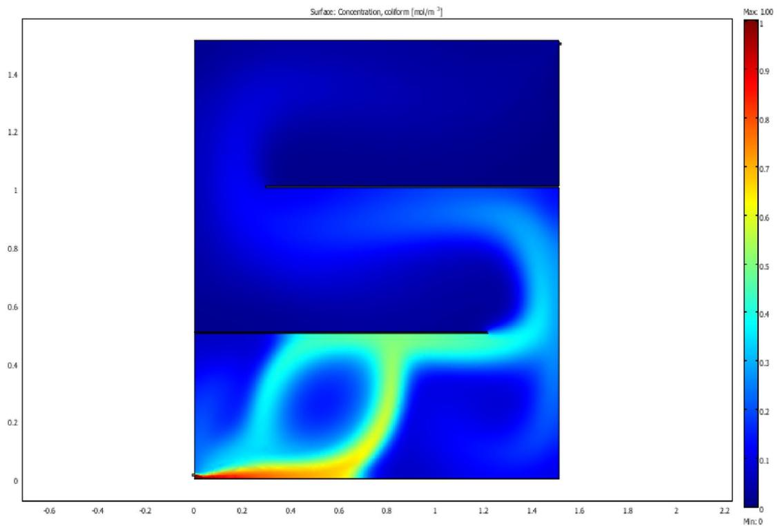
**Figure 4.65** MOGA-II optimal faecal coliform removal design with least cost for even baffle longitudinal arrangement in maturation reactor
