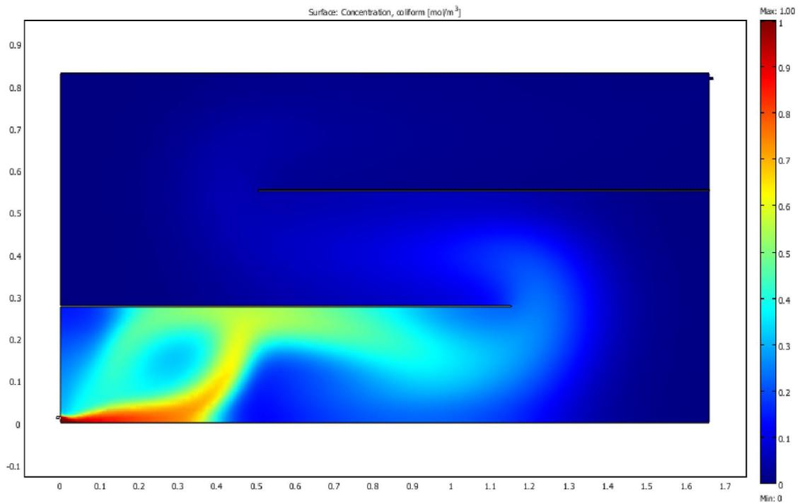
**Figure 4.70** SIMPLEX sensitivity optimal faecal coliform removal design with least cost for longitudinal baffle arrangement in facultative reactor ( $k = 13.686$ )
