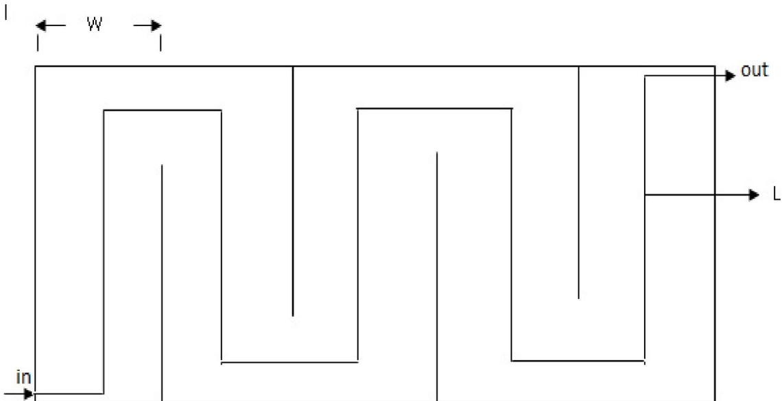
**Figure 3.9** Description of length to width ratio for the laboratory-scale model
