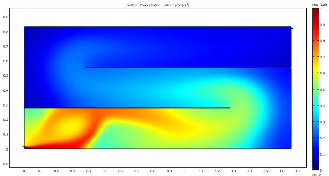
**Figure 4.76** SIMPLEX sensitivity optimal faecal coliform removal design with least cost for longitudinal baffle arrangement in facultative reactor ( $k = 4.562$ )
