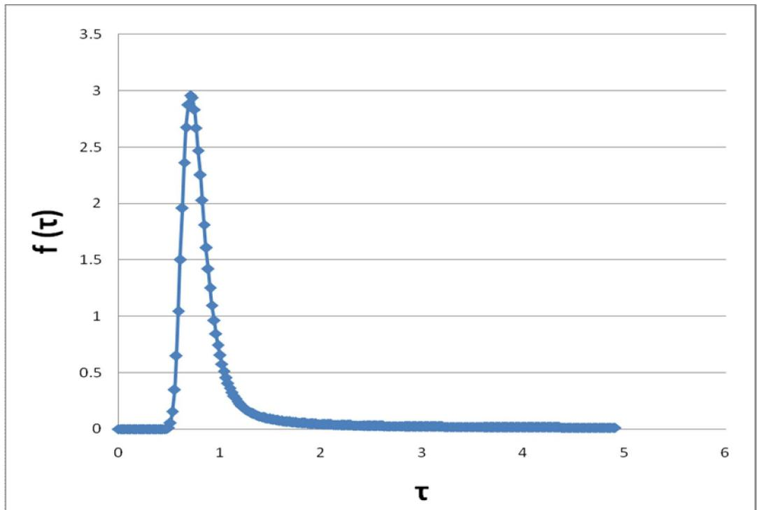
**Figure 4.18** Residence time distribution curve for longitudinal 4-baffle 70% pond width Maturation reactor
