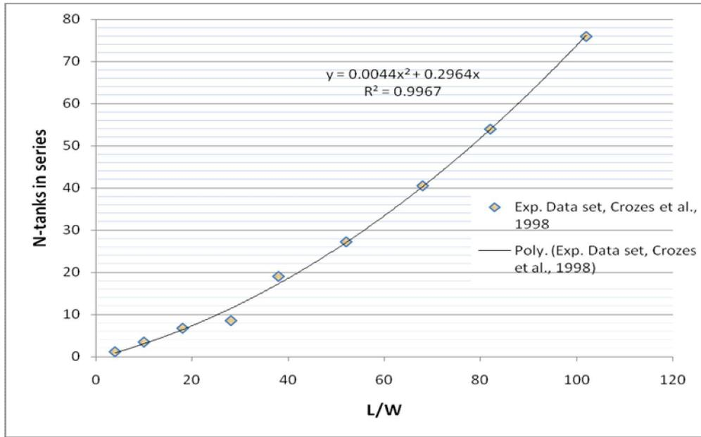
**Figure 3.8** Data conversion for reactor length to width ratio to N for N-tanks in series model. Source: Ducoste et al., 2001.
