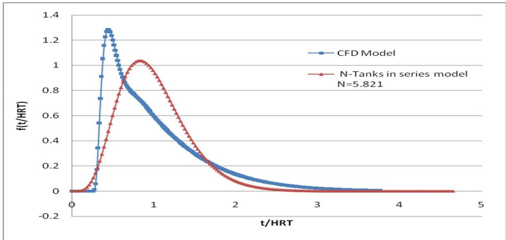
**Figure 4.30** Comparison of residence time density curves in 4-baffles, 80% pond width Maturation reactor for CFD and N-tanks in series models.
