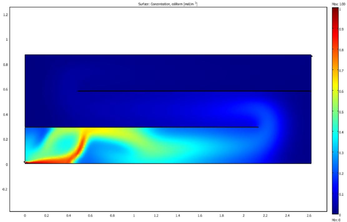
**Figure 4.47** SIMPLEX optimal faecal coliform removal design for combination of even and odd longitudinal baffle arrangement in maturation reactor
