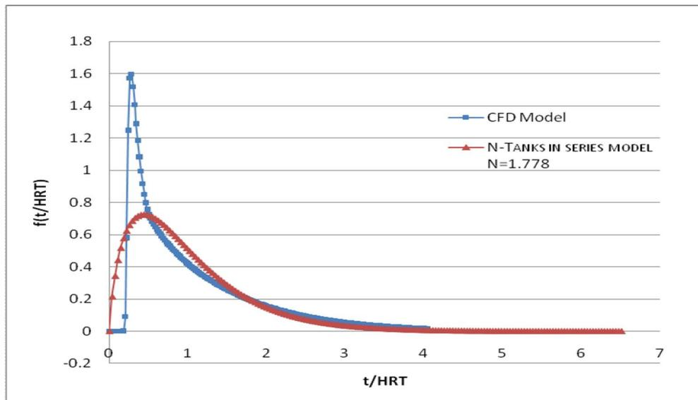
**Figure 4.20** Comparison of residence time density curves in 2-baffles, 70% pond width Facultative reactor for CFD and N-tanks in series models.
