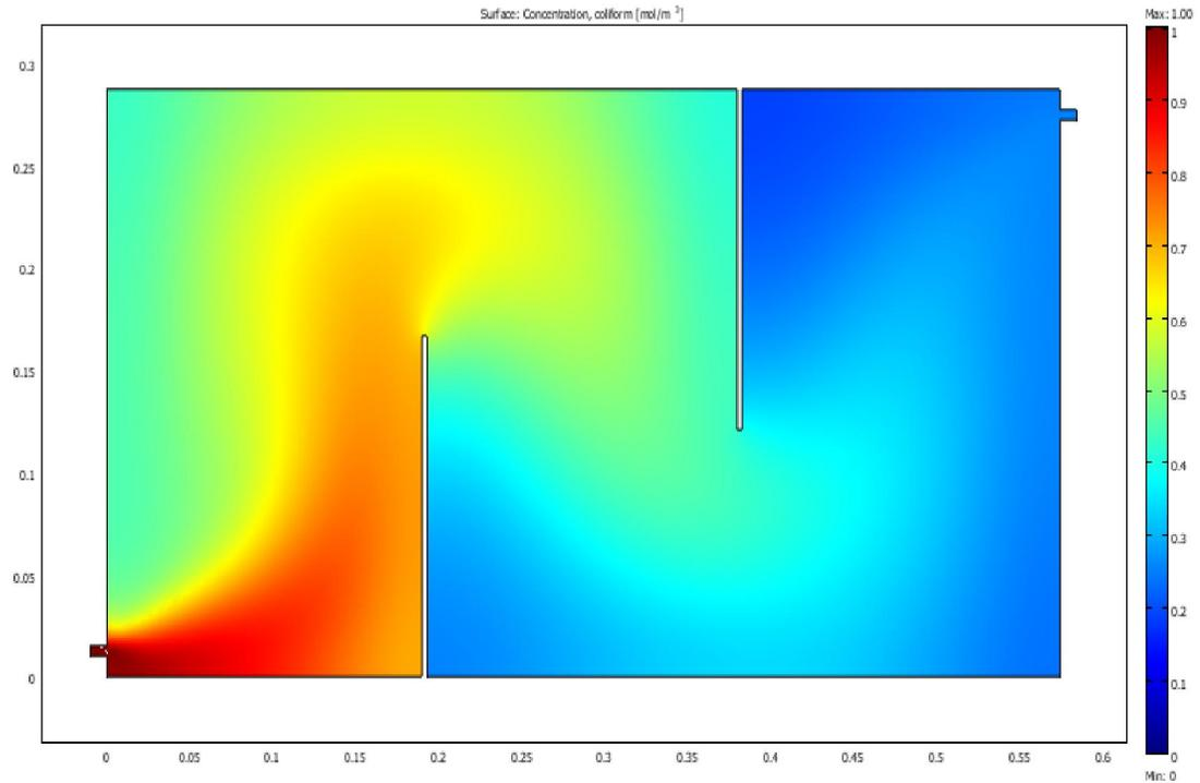
**Figure 4.54** MOGA-II optimal faecal coliform removal design with least cost for even baffle transverse arrangement in anaerobic reactor
