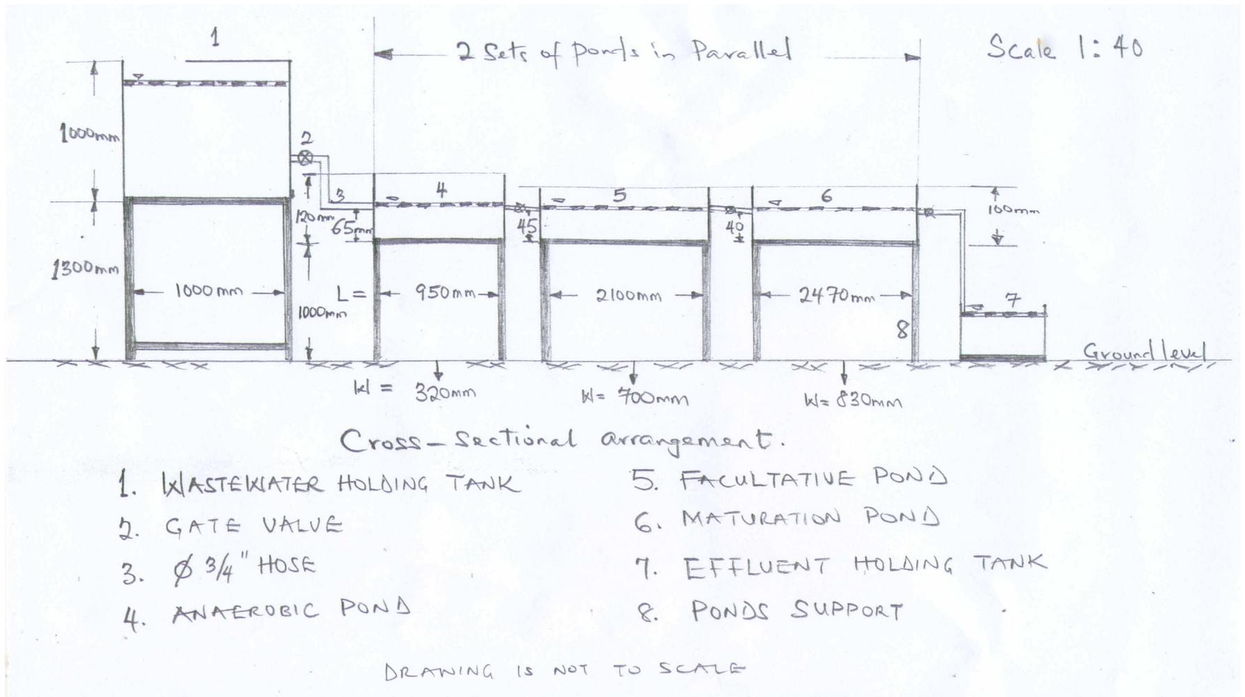
**Fig. 3.3 A sketch of the laboratory-scale WSP and operating conditions.**
