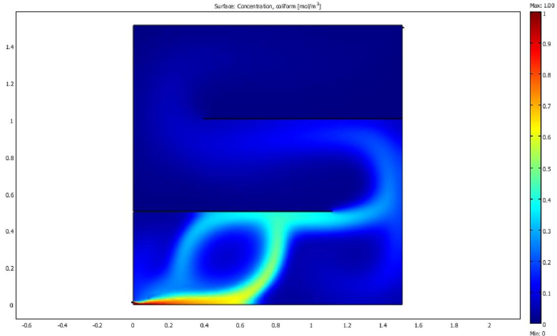
**Figure 4.83** MOGA II sensitivity analysis optimal faecal coliform removal design with least cost for longitudinal baffle arrangement in maturation reactor ( $k = 13.686$ )
