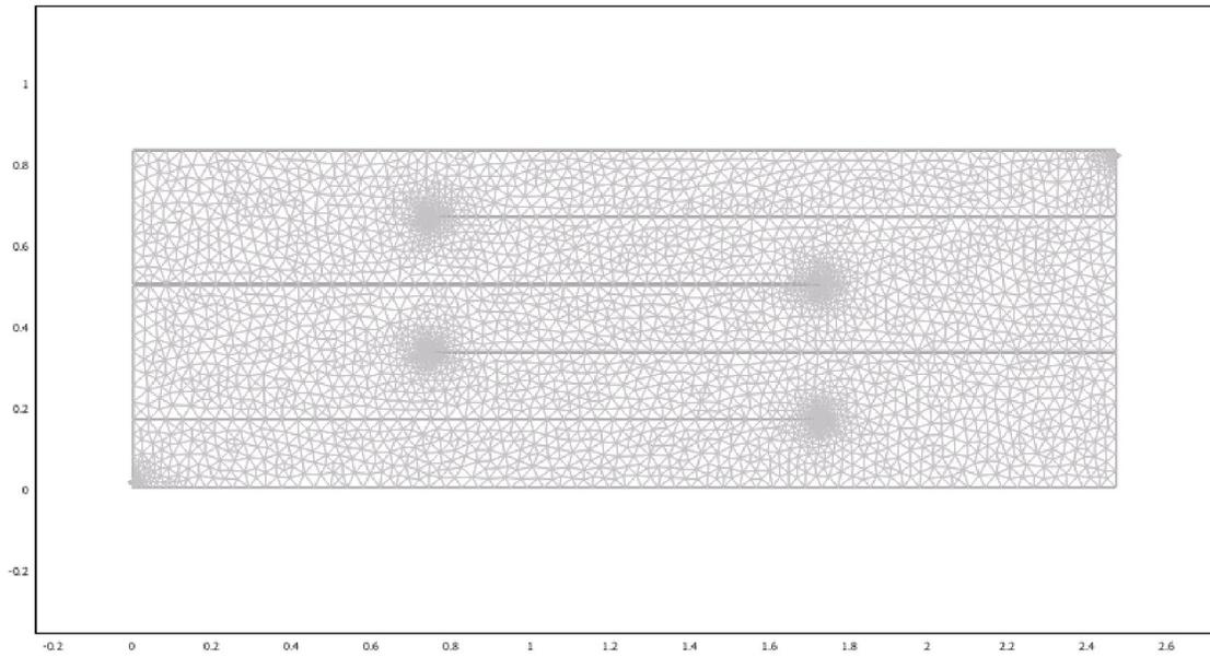
**Figure 3.23** Mesh structure in a 4 baffled 70% Longitudinal Maturation
