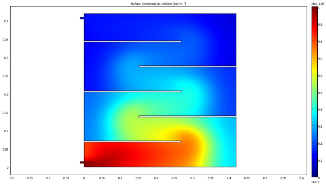
**Figure 4.69** SIMPLEX sensitivity optimal faecal coliform removal design with least cost for longitudinal baffle arrangement in anaerobic reactor ( $k = 13.686$ )
