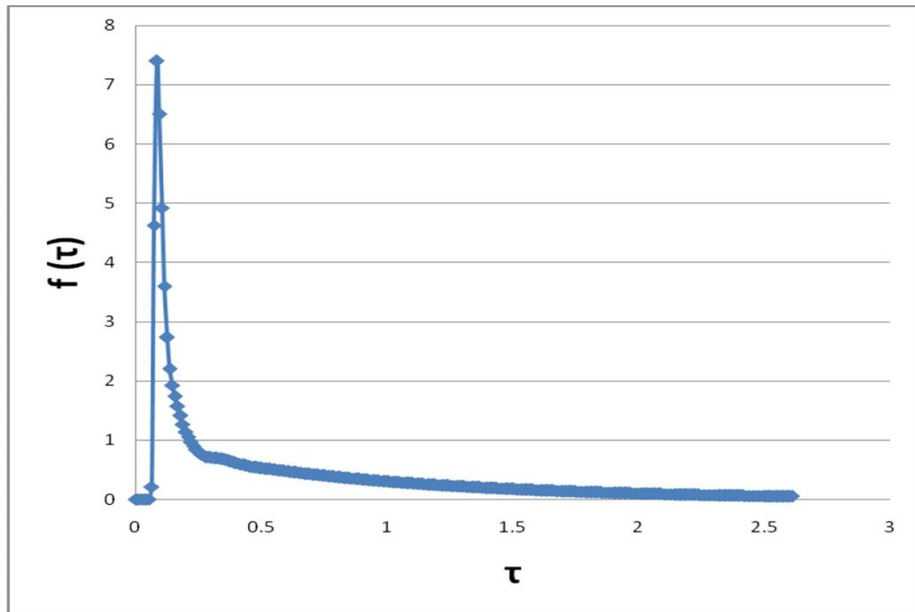
**Figure 4.5** Residence time distribution curve for un baffled maturation reactor
