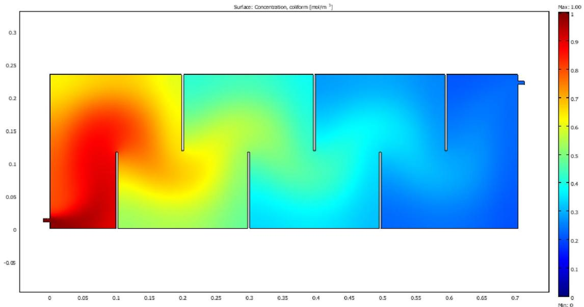
**Figure 4.40** SIMPLEX maximum faecal coliform removal design for combination of even and odd transverse baffle arrangement in anaerobic reactor
