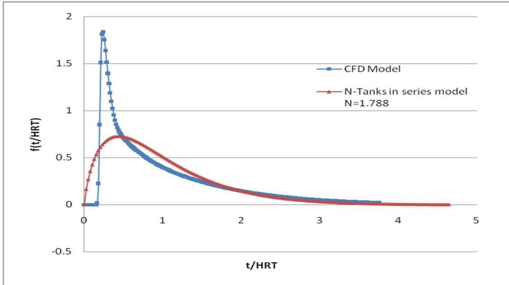
**Figure 4.23** Comparison of residence time density curves in 2-baffles, 70% pond width Maturation reactor for CFD and N-tanks in series models
