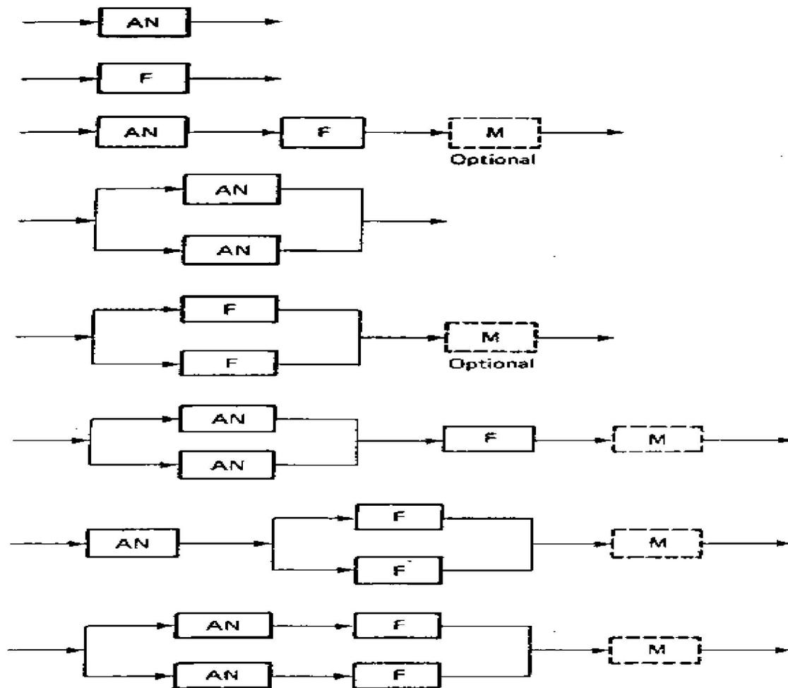
**Figure 2.1** Waste stabilization pond configurations: AN = anaerobic pond; F = facultative pond; M = maturation pond (Pescod and Mara, 1988).
