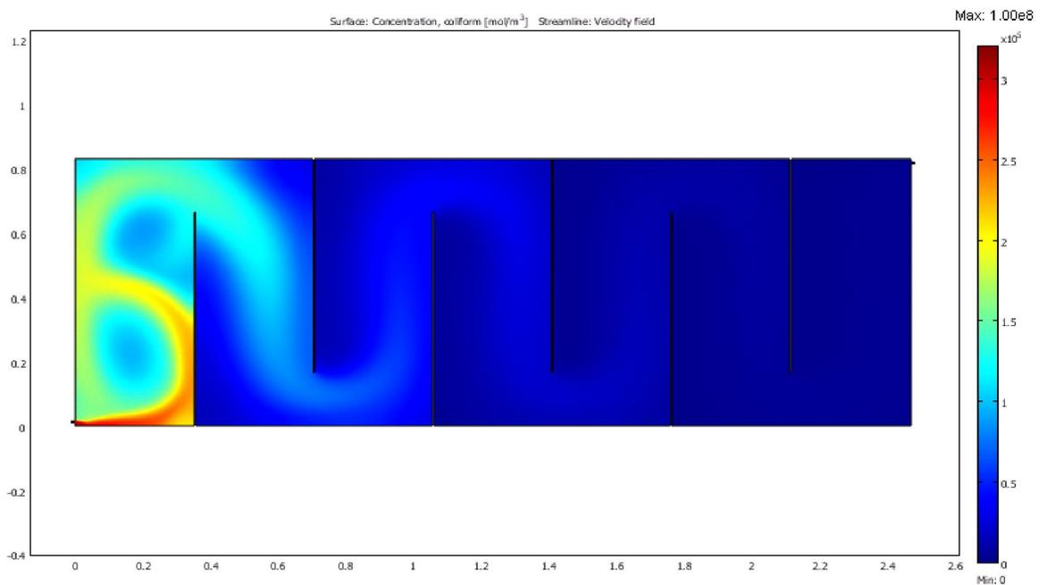
**Figure 4.37** Faecal coliform inactivation in a transverse 4-baffle 80% pond width maturation reactor
