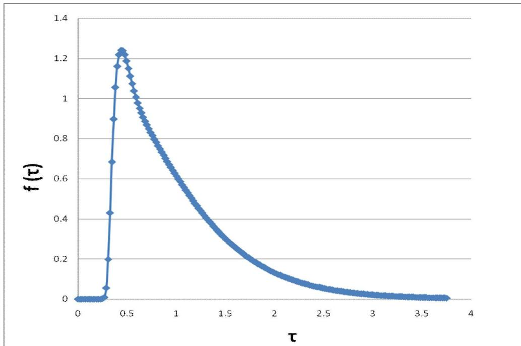
**Figure 4.10** Residence time distribution curve for transverse 4-baffle with 70% pond width Facultative reactor
