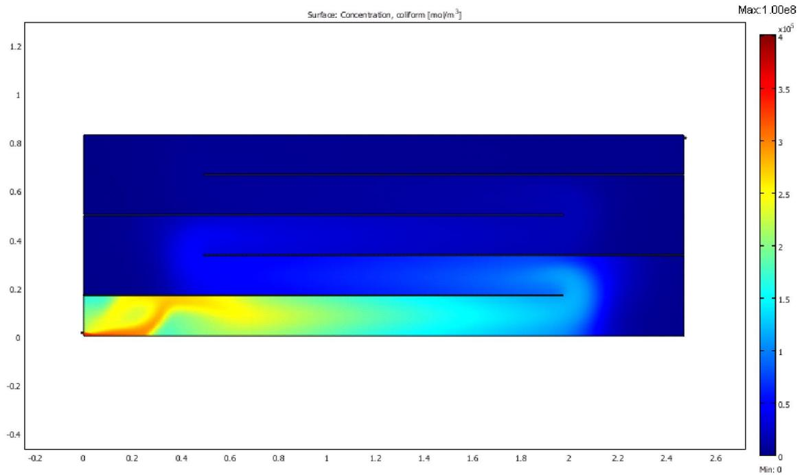
**Figure 4.36** Faecal coliform inactivation in a longitudinal 4-baffle 80% pond width maturation reactor
