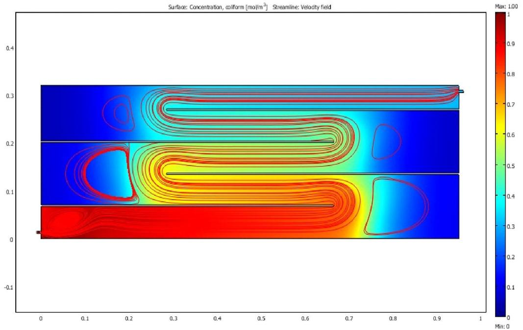
**Figure 4.15** Velocity streamline and coliform inactivation for longitudinal 70% pond width anaerobic reactor.
