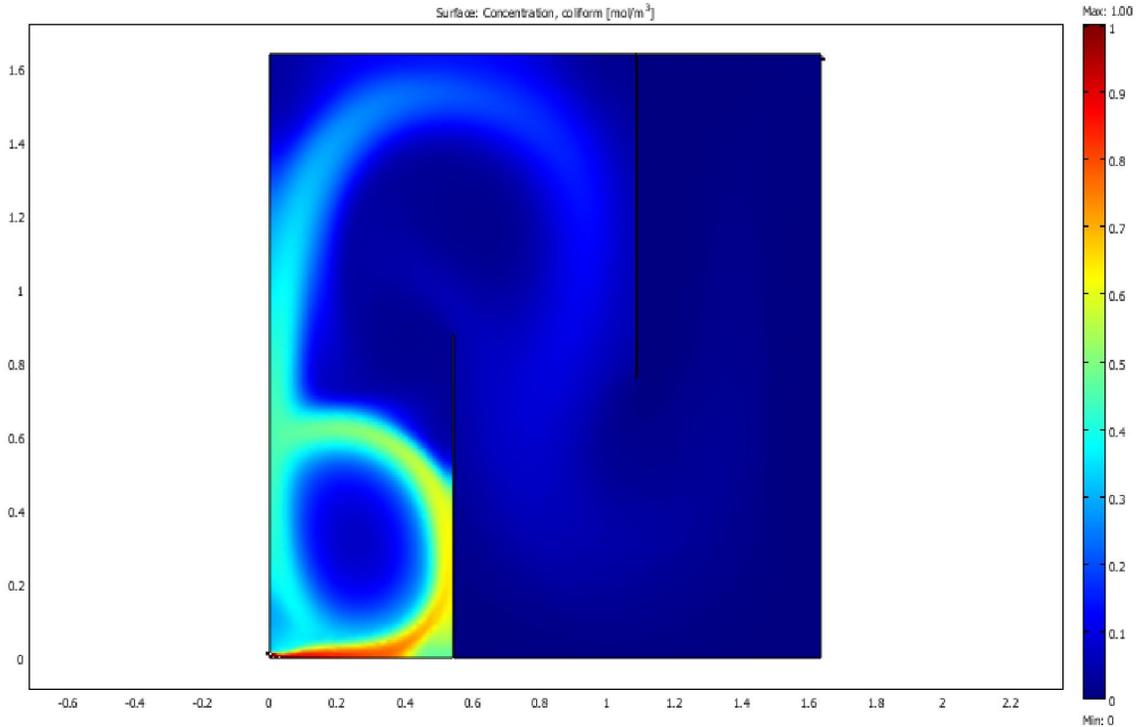
**Figure 4.80** MOGA II sensitivity analysis optimal faecal coliform removal design with least cost for transverse baffle arrangement in maturation reactor ( $k = 13.686$ )
