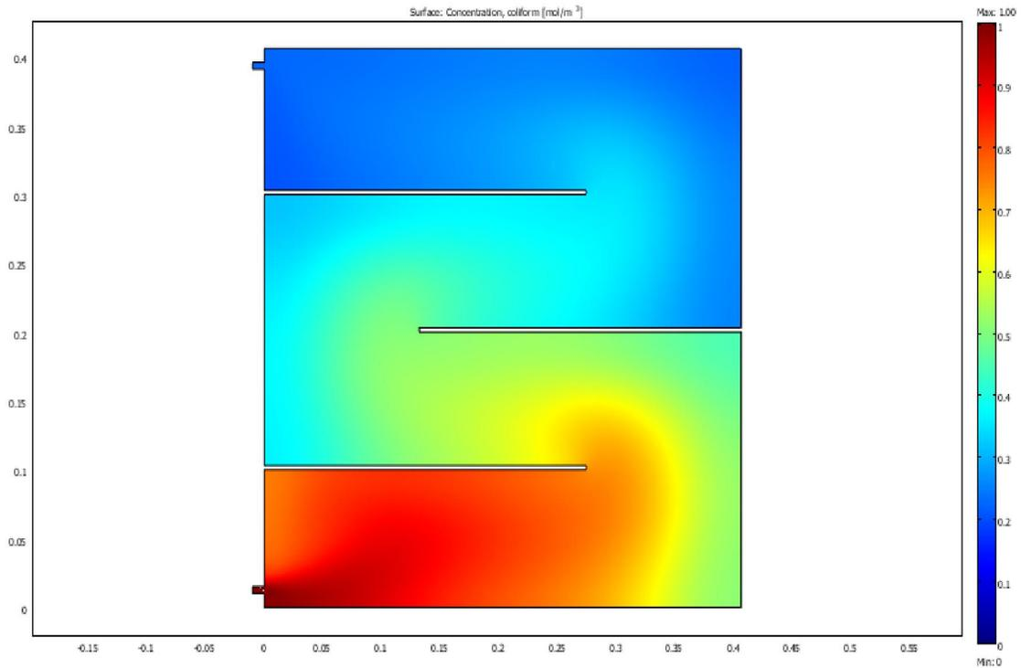
**Figure 4.62** MOGA-II optimal faecal coliform removal design with least cost for even baffle longitudinal arrangement in anaerobic reactor
