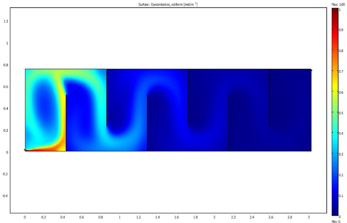
**Figure 4.42** SIMPLEX optimal faecal coliform removal design with least cost for combination of even and odd transverse baffle arrangement in maturation reactor
