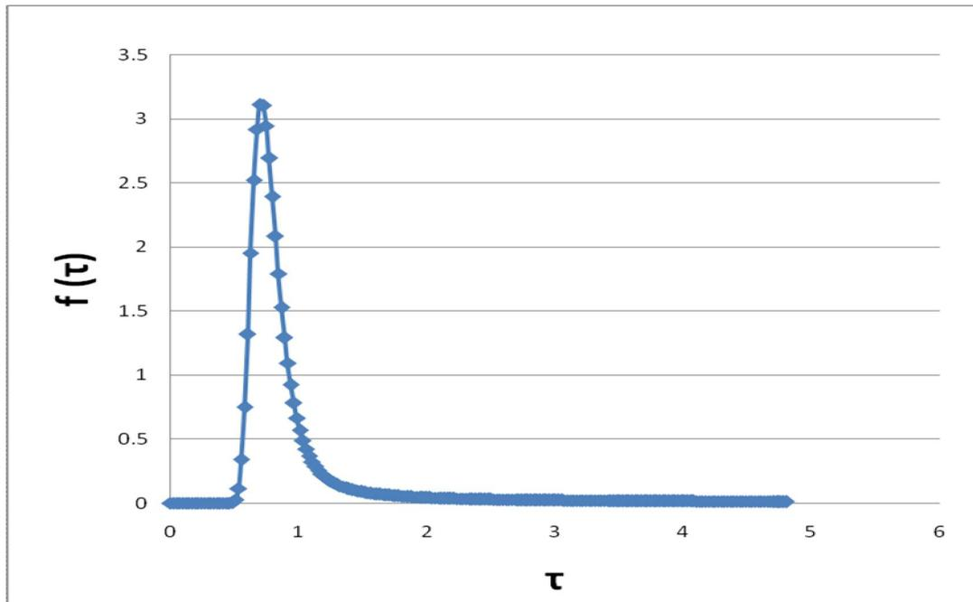
**Figure 4.16** Residence time distribution curve for longitudinal 4-baffle with 70% pond width Facultative reactor
