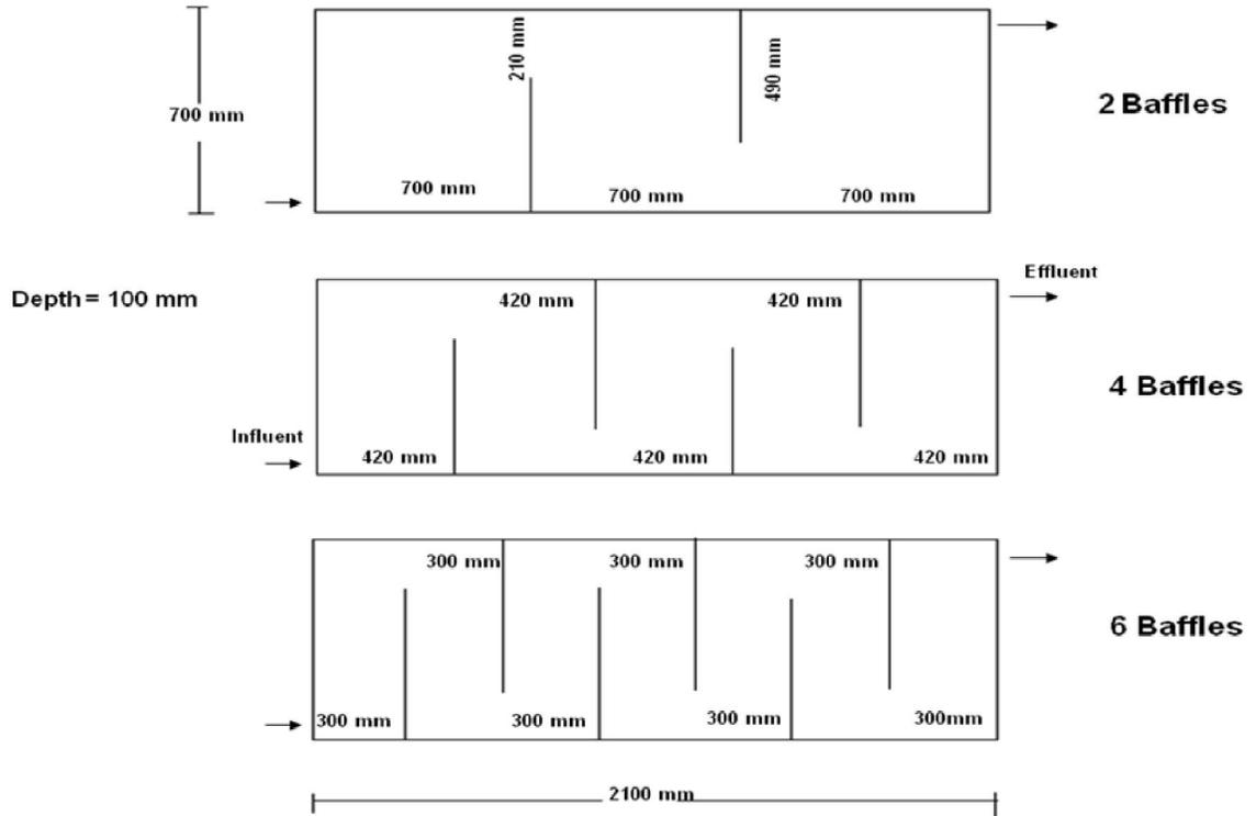
**Figure 3.6** Different baffle arrangements with 70% pond width facultative reactors
