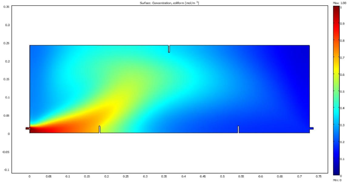
**Figure 4.66** SIMPLEX optimal faecal coliform removal design with least cost for transverse baffle arrangement in anaerobic reactor ( $k = 13.686$ )
