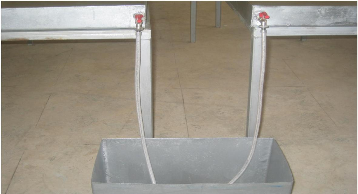
**Plate 3.16** outlet structures connected to two pieces of ½ inch hoses for effluent discharge
