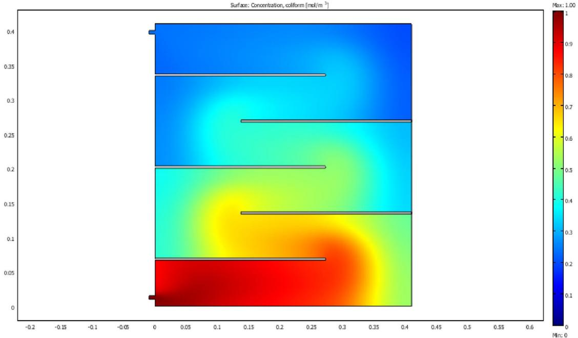
**Figure 4.44** SIMPLEX optimal faecal coliform removal design with least cost for combination of even and odd longitudinal baffle arrangement in anaerobic reactor
