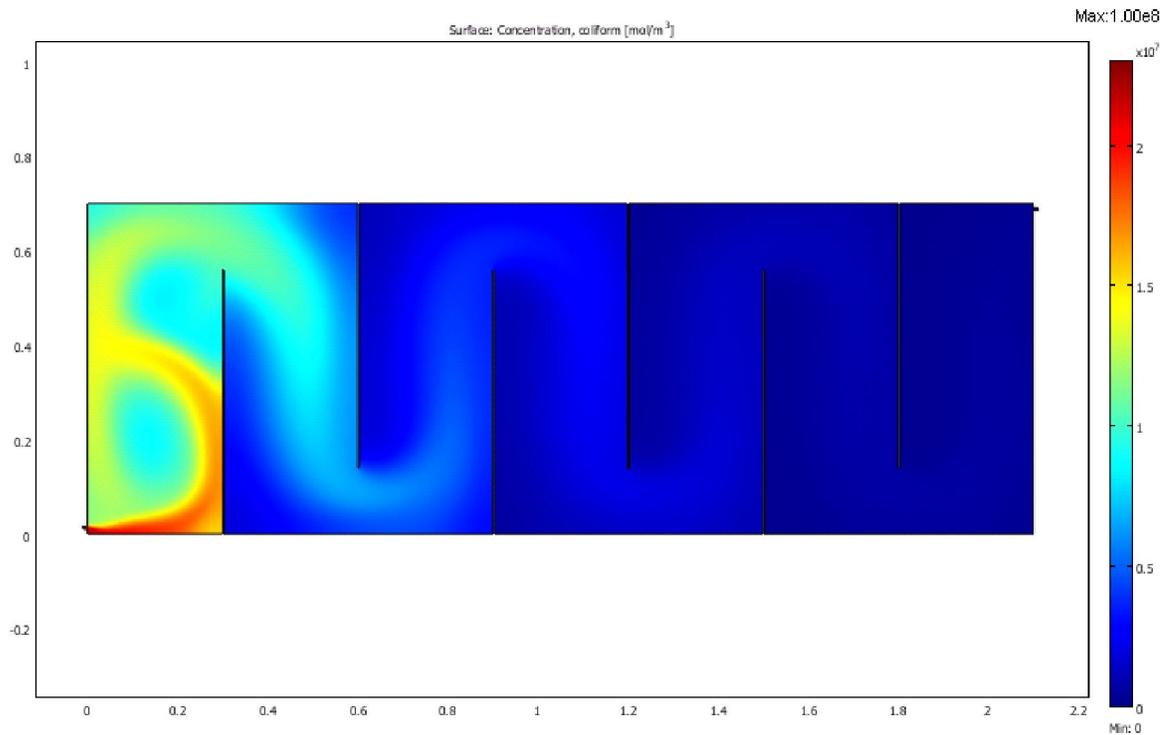
**Figure 4.35** Faecal coliform inactivation in a transverse 6-baffle 80% pond width facultative reactor
