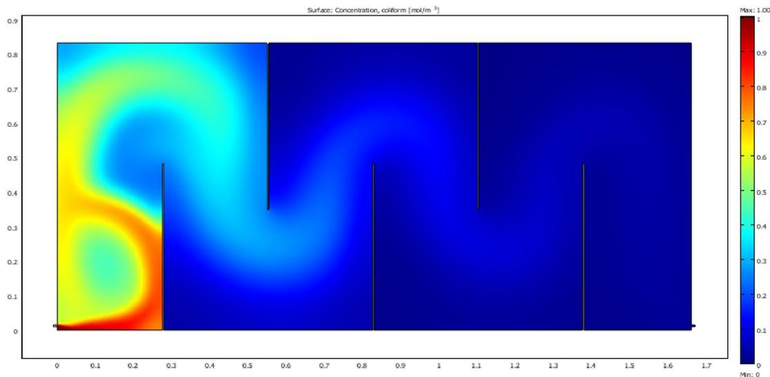
**Figure 4.41** SIMPLEX optimal faecal coliform removal design with least cost for the combination of even and odd transverse baffle arrangement in facultative reactor
