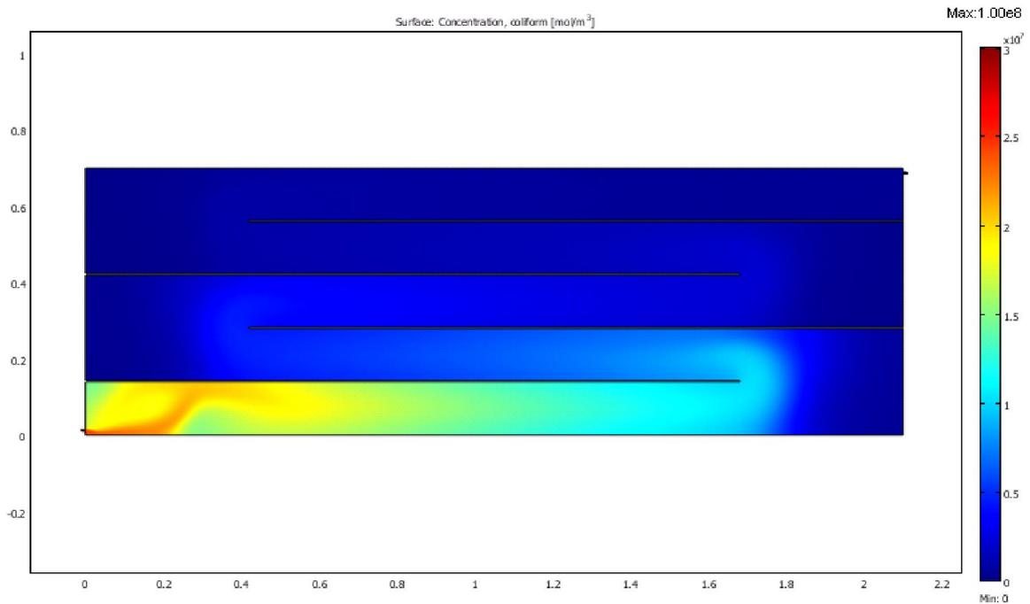
**Figure 4.34** Faecal coliform inactivation in a longitudinal 4-baffle 80% pond width facultative reactor
