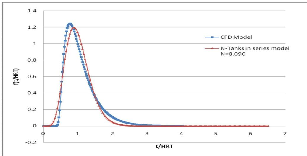
**Figure 4.22** Comparison of residence time density curves in 6-baffles, 70% pond width Facultative reactor for CFD and N-tanks in series models
