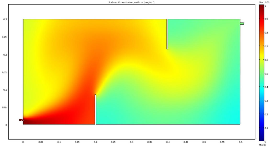
**Figure 4.84** MOGA II sensitivity analysis optimal faecal coliform removal design with least cost for transverse baffle arrangement in anaerobic reactor ( $k = 4.562$ )
