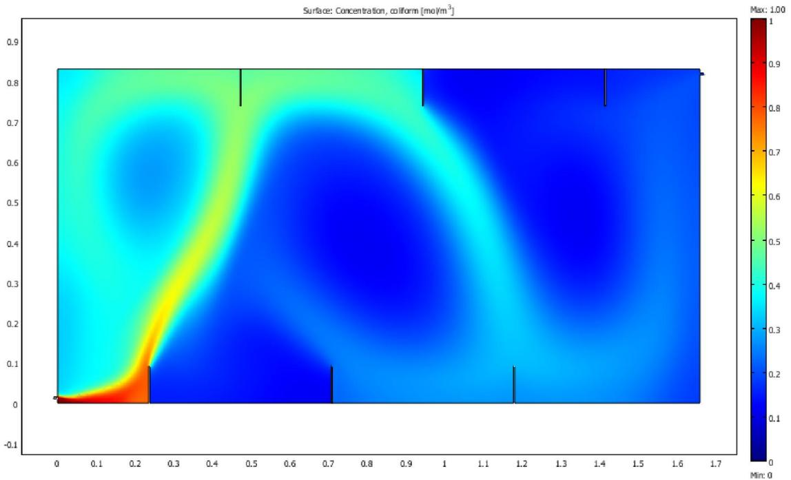
**Figure 4.85** MOGA II sensitivity analysis optimal faecal coliform removal design with least cost for transverse baffle arrangement in facultative reactor ( $k = 4.562$ )
