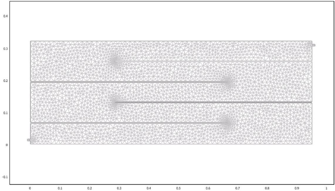
**Figure 3.19** Mesh structure in a 4 baffled 70% Longitudinal Anaerobic reactor
