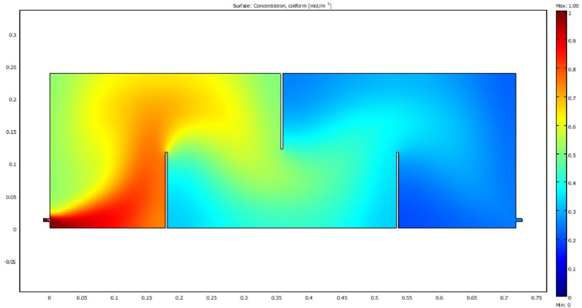
**Figure 4.39** SIMPLEX optimal faecal coliform removal design with least cost for the combination of even and odd transverse baffle arrangement in anaerobic reactor
