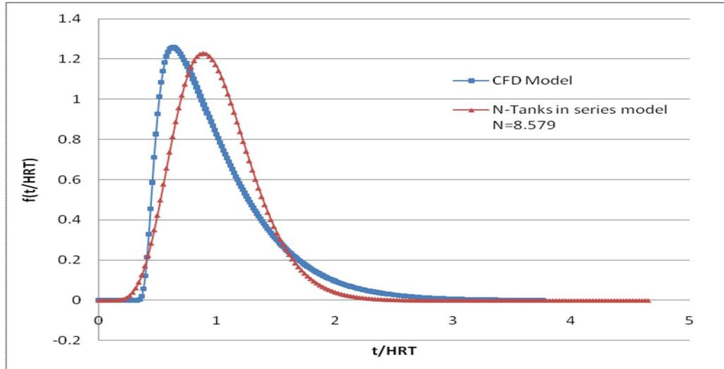
**Figure 4.31** Comparison of residence time density curves in 6-baffles, 80% pond width Facultative reactor for CFD and N-tanks in series models.
