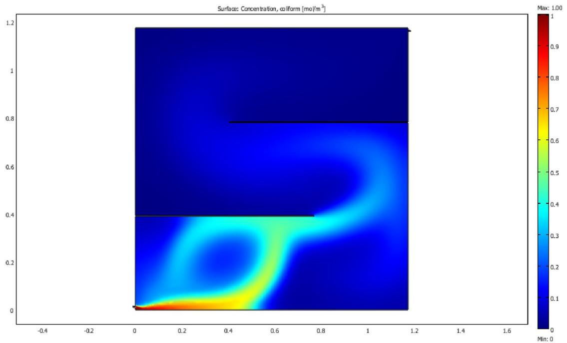
**Figure 4.82** MOGA II sensitivity analysis optimal faecal coliform removal design with least cost for longitudinal baffle arrangement in facultative reactor ( $k = 13.686$ )
