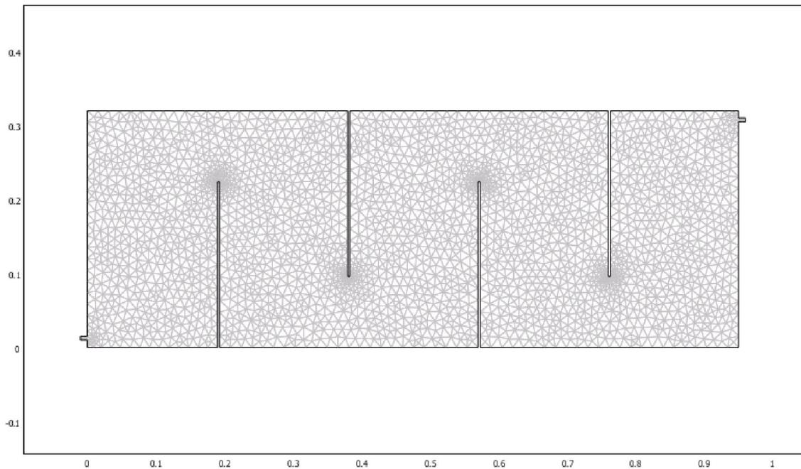
**Figure 3.18** Mesh structure in a 4 baffled 70% Transverse Anaerobic reactor
