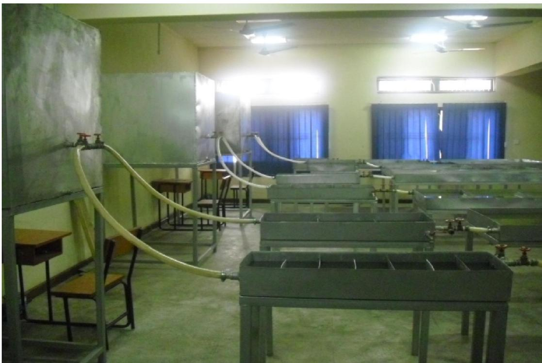
**Plate 3.14** Two 25-mm PVC hoses linked with the T-connector
