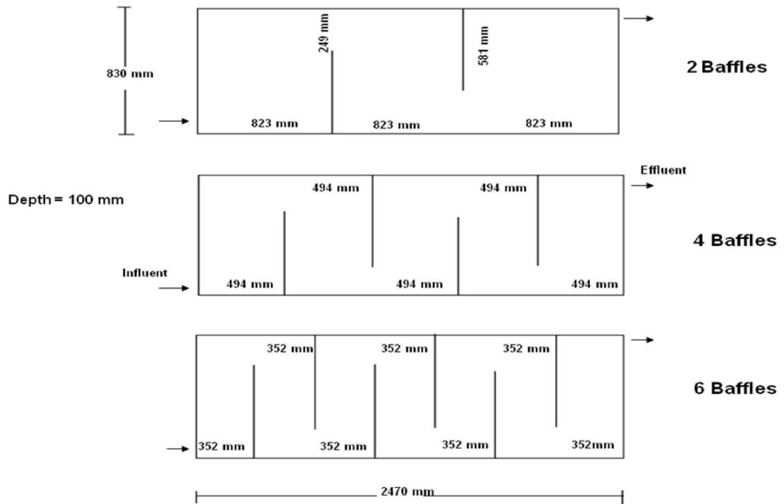
**Figure 3.7** Different baffle arrangements with 70% pond width maturation reactors
