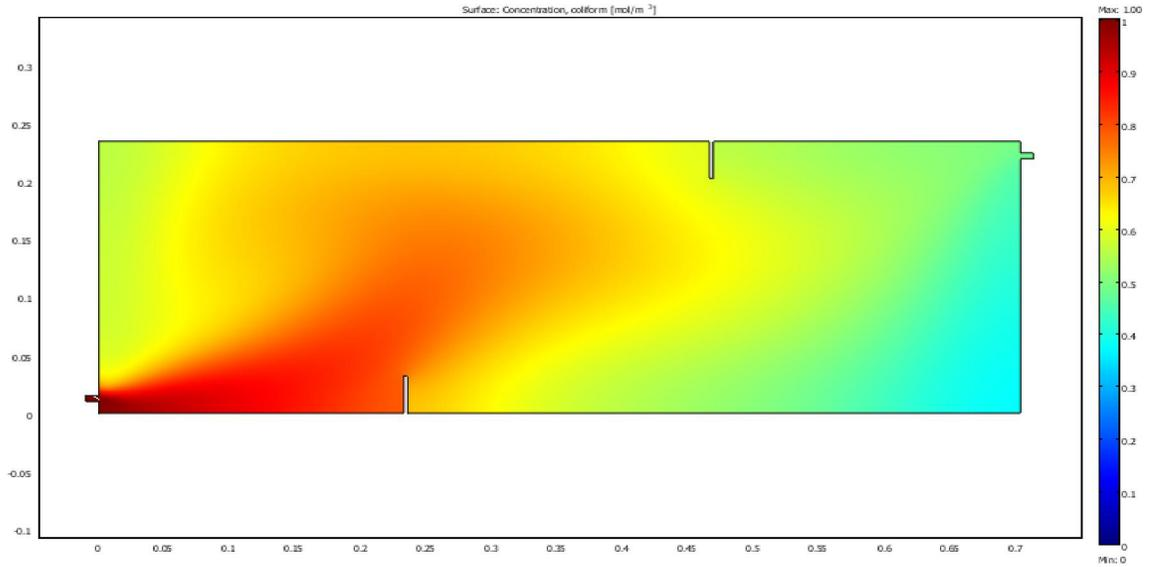
**Figure 4.72** SIMPLEX sensitivity optimal faecal coliform removal design with least cost for transverse baffle arrangement in anaerobic reactor ( $k = 4.562$ )
