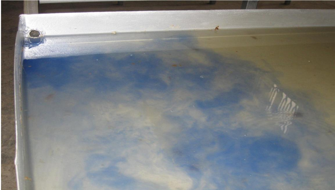
**Plate 3.18** Tracer chemical diluting with the wastewater before getting to the outlet.
