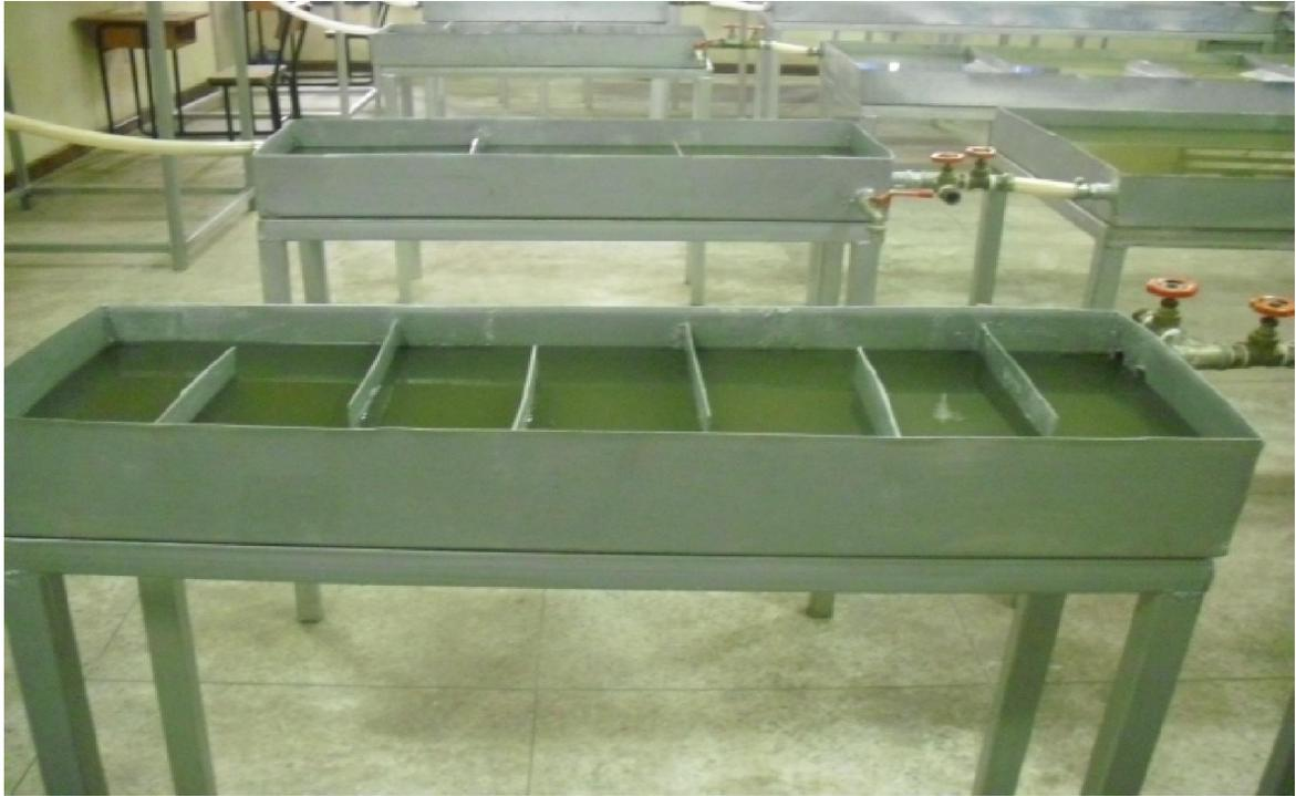
**Plate 3.10** Laboratory-scaled anaerobic reactors
