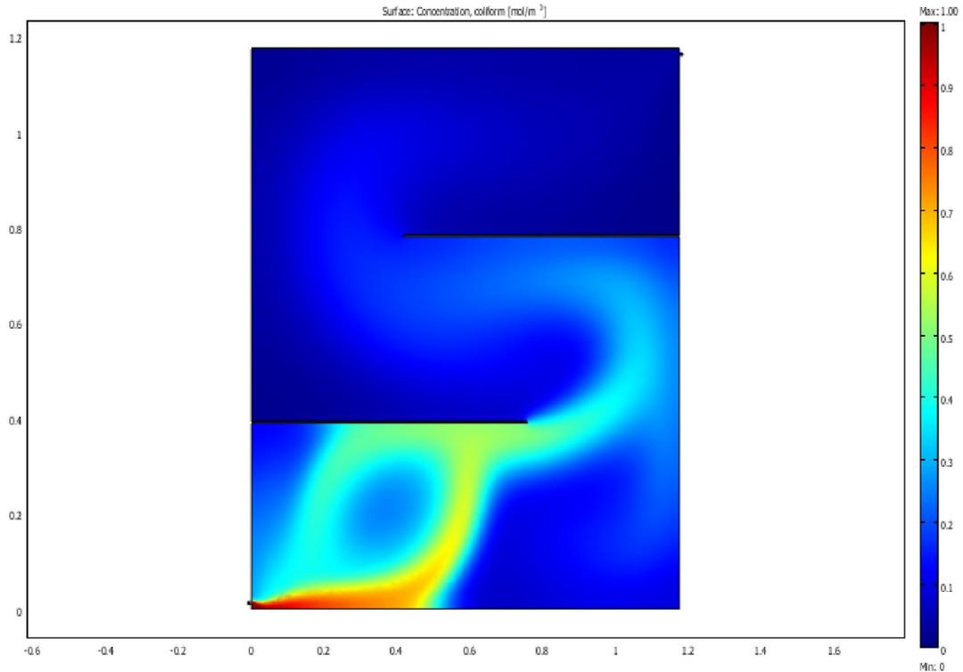
**Figure 4.63** MOGA-II optimal faecal coliform removal design with least cost for even baffle longitudinal arrangement in facultative reactor
