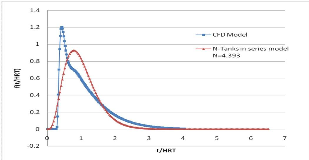
**Figure 4.27** Comparison of residence time density curves in 4-baffles, 80% pond width Facultative reactor for CFD and N-tanks in series models
