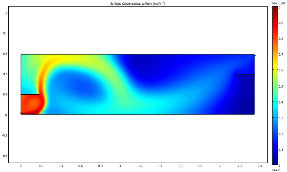
**Figure 4.88** MOGA II sensitivity analysis optimal faecal coliform removal design with least cost for longitudinal baffle arrangement in facultative reactor ( $k = 4.562$ )
