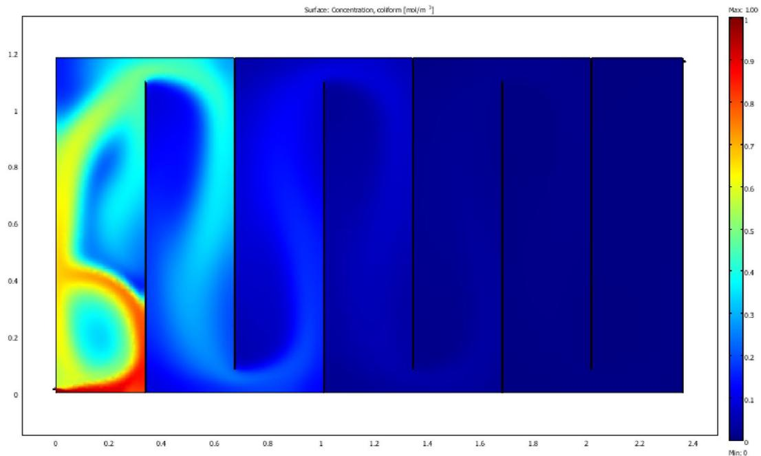
**Figure 4.58** MOGA-II maximum faecal coliform removal design for even baffle transverse arrangement in maturation reactor
