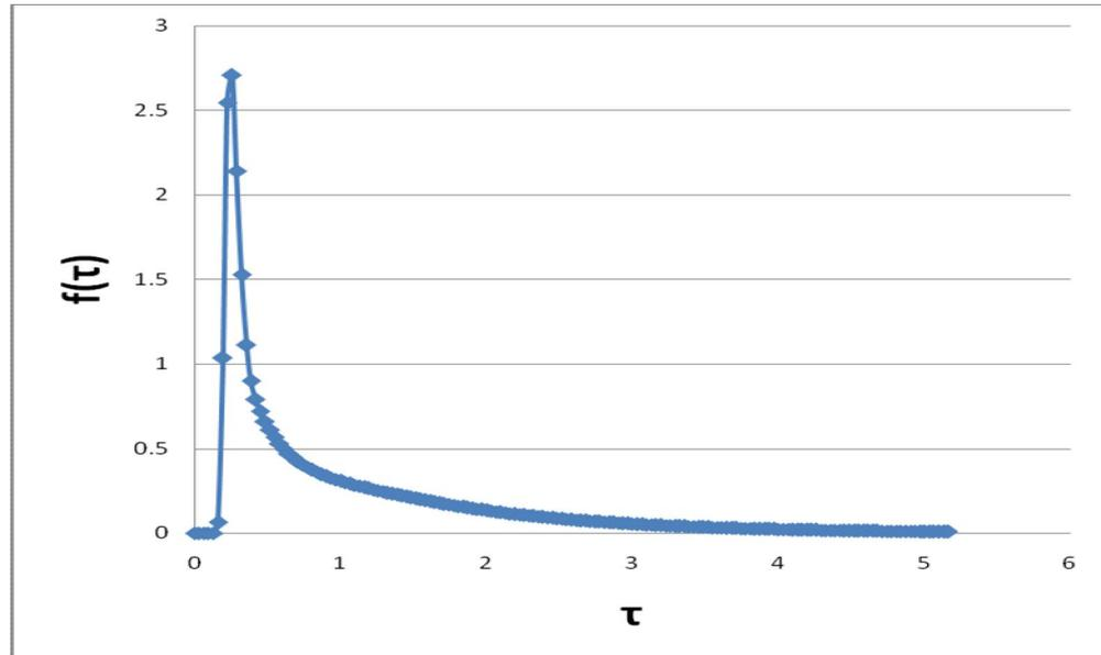
**Figure 4.1** Residence time distribution curve for un baffled anaerobic reactor
