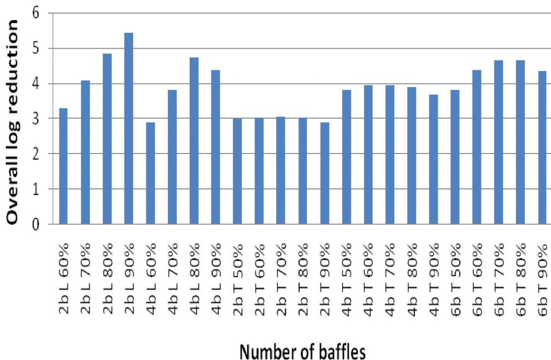
**Figure 4.7:** Overall log reductions for the WSP system over a range of baffle lengths tested
