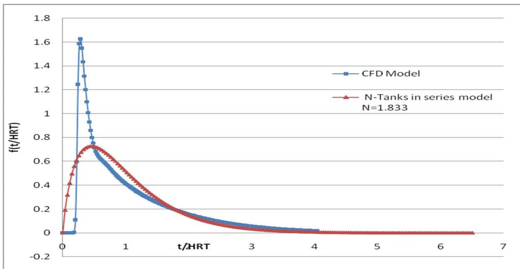
**Figure 4.26** Comparison of residence time density curves in 2-baffles, 80% pond width Facultative reactor for CFD and N-tanks in series models
