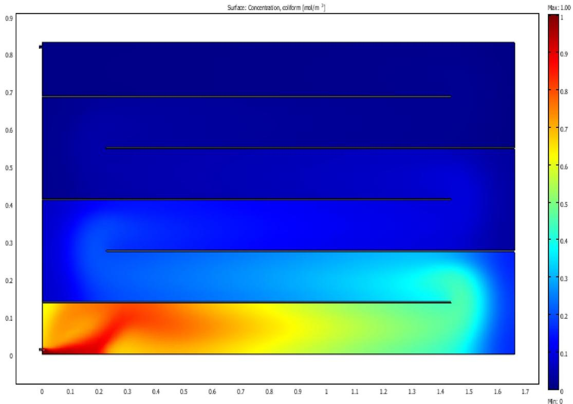
**Figure 4.64** MOGA-II maximum faecal coliform removal design for even baffle longitudinal arrangement in facultative reactor
