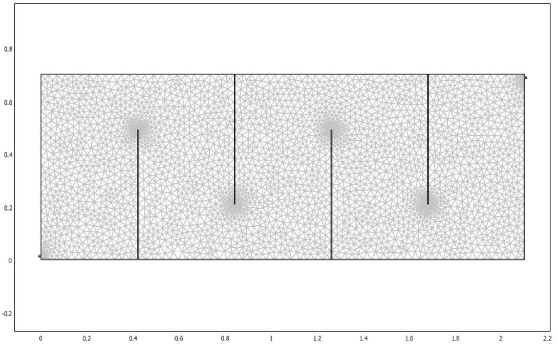
**Figure 3.20** Mesh structure in a 4 baffled 70% Transverse Facultative reactor
