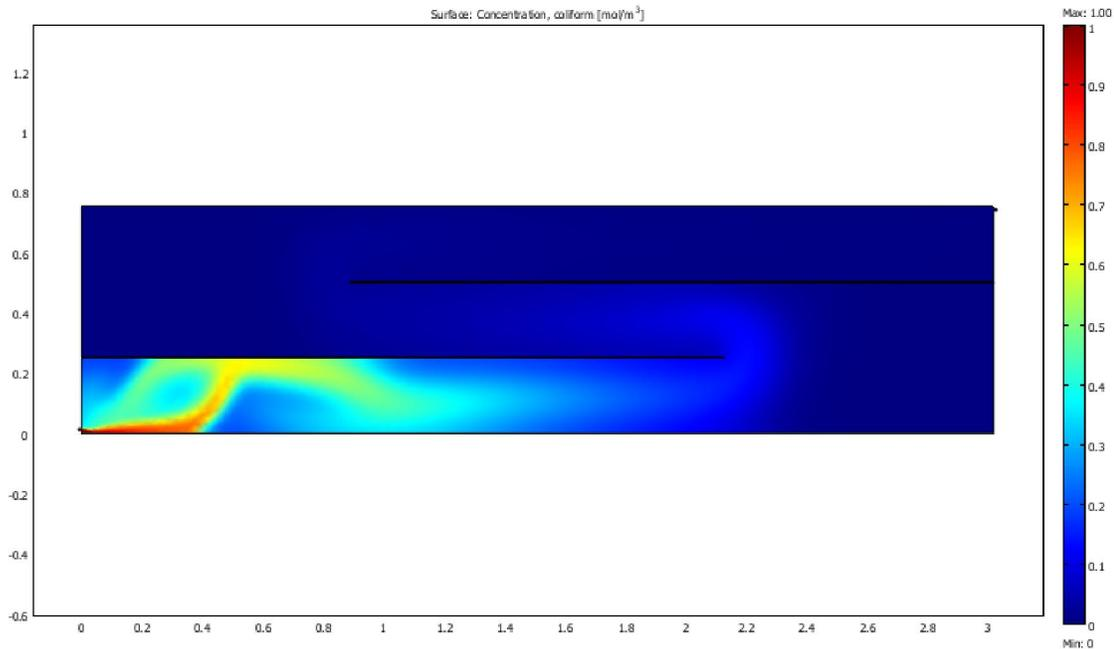
**Figure 4.71** SIMPLEX sensitivity optimal faecal coliform removal design with least cost for longitudinal baffle arrangement in maturation reactor ( $k = 13.686$ )
