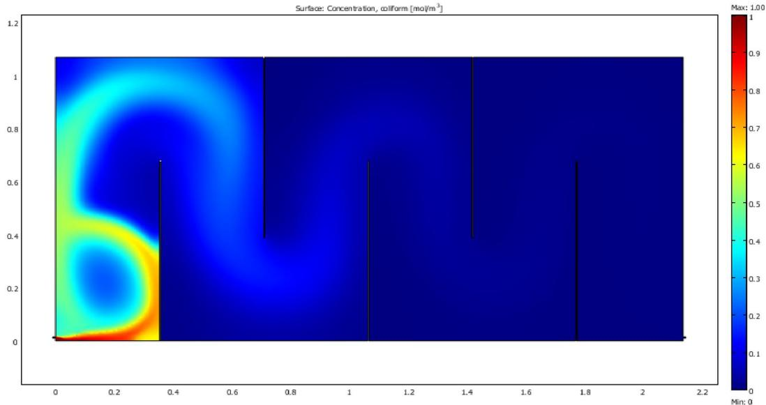
**Figure 4.68** SIMPLEX sensitivity optimal faecal coliform removal design with least cost for transverse baffle arrangement in maturation reactor ( $K= 13.686$ )
