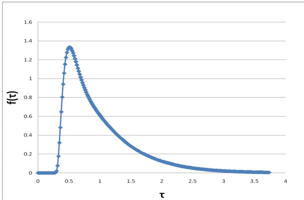
**Figure 4.12** Residence time distribution curve for transverse 4-baffle with 70% Pond width Maturation reactor
