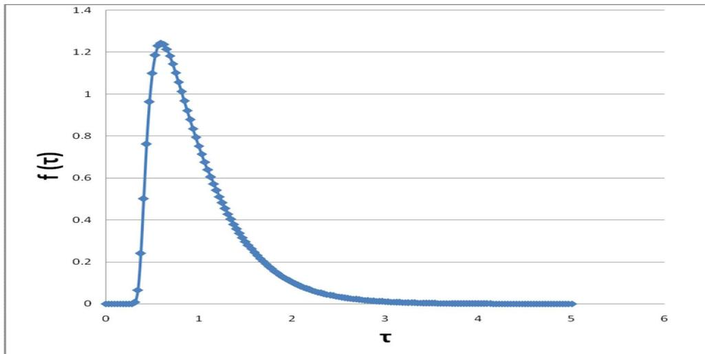
**Figure 4.8** Residence time distribution curve for transverse 4-baffle with 70% Pond width anaerobic reactor
