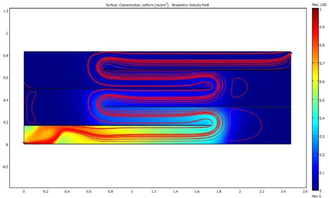
**Figure 4.19** Velocity streamline and coliform inactivation for longitudinal 4-baffle 70% pond width maturation reactor
