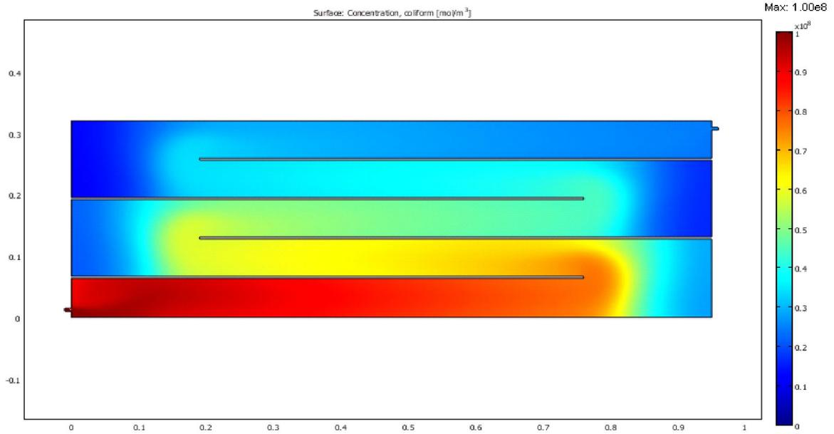
**Figure 4.32** Faecal coliform inactivation in a longitudinal 4-baffle 80% pond width anaerobic reactor
