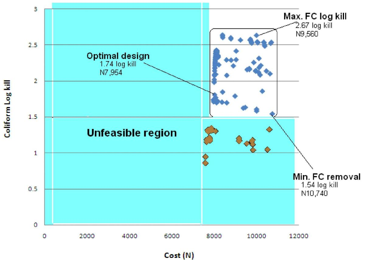
**Figure 4.53** Trade off plot for Maturation Transverse design space.
