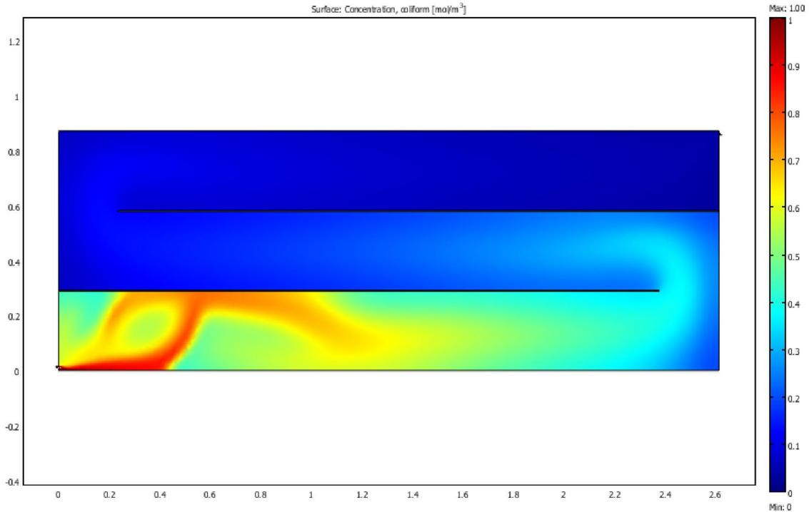
**Figure 4.77** SIMPLEX sensitivity optimal faecal coliform removal design with least cost for longitudinal baffle arrangement in maturation reactor ( $k = 4.562$ )
