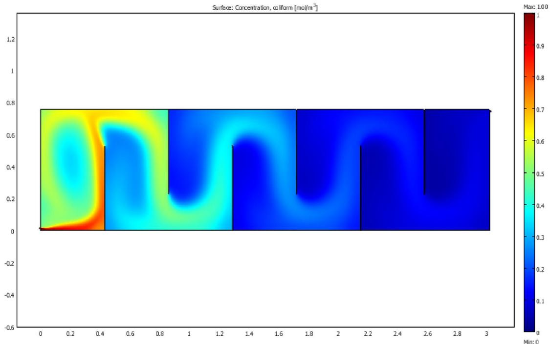
**Figure 4.74** SIMPLEX sensitivity optimal faecal coliform removal design with least cost for transverse baffle arrangement in maturation reactor ( $k = 4.562$ )
