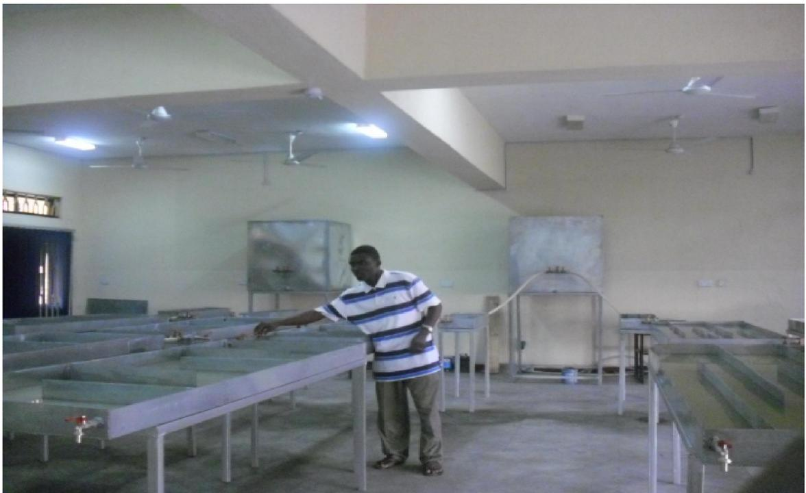
**Plate 3.9** Inlet-outlet alternation of laboratory-scale WSP
