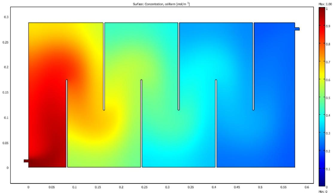
**Figure 4.55** MOGA-II maximum faecal coliform removal design for even baffle transverse arrangement in anaerobic reactor
