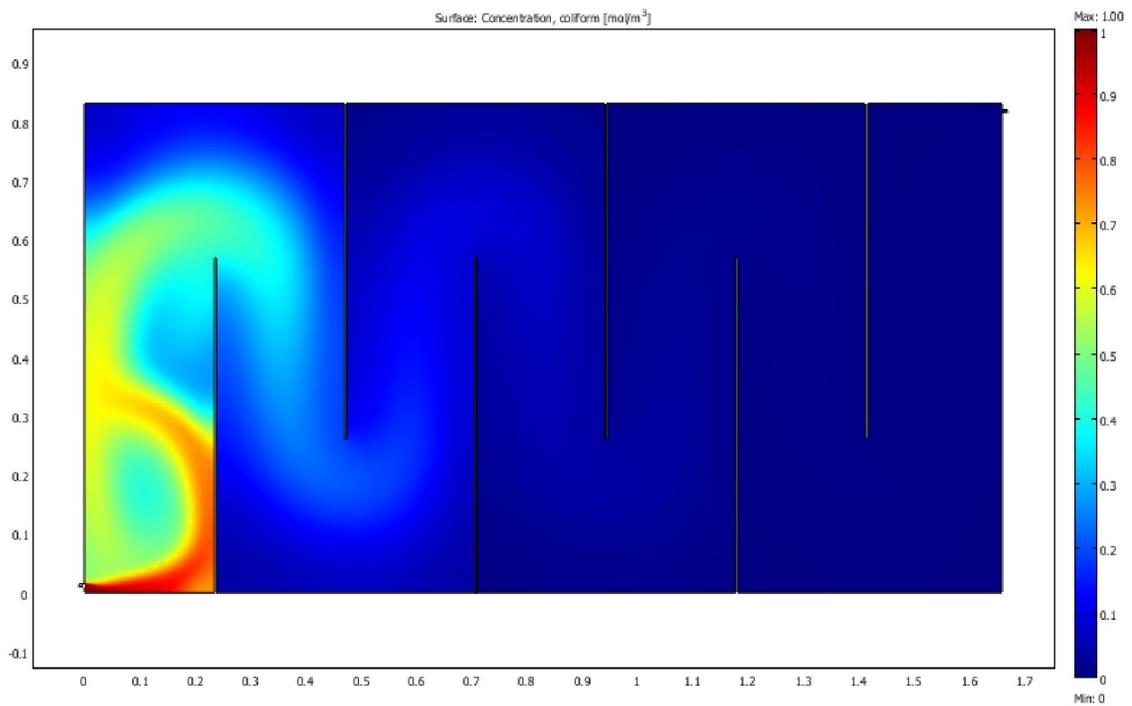
**Figure 4.67** SIMPLEX sensitivity optimal faecal coliform removal design with least cost for transverse baffle arrangement in facultative reactor ( $k = 13.686$ )
