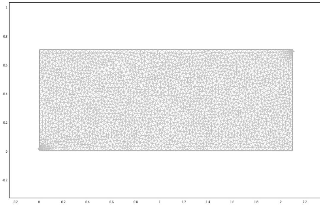
**Figure 3.11** Triangular meshes for the model facultative reactor
