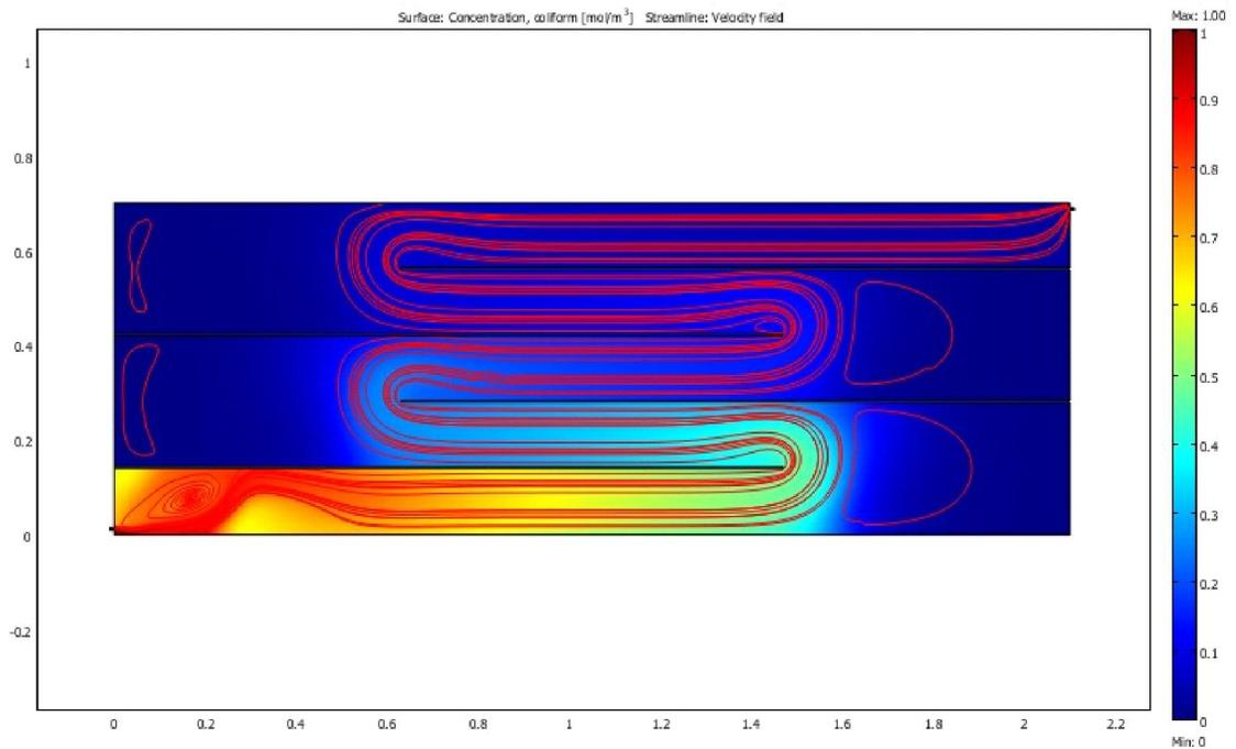
**Figure 4.17** Velocity streamline and coliform inactivation for longitudinal 4 baffle 70% pond width facultative reactor
