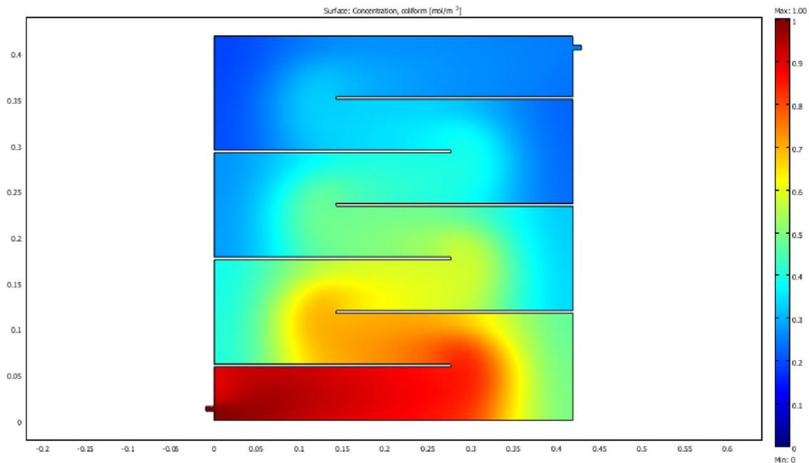
**Figure 4.45** SIMPLEX minimum faecal coliform removal design for combination of even and odd longitudinal baffle arrangement in anaerobic reactor
