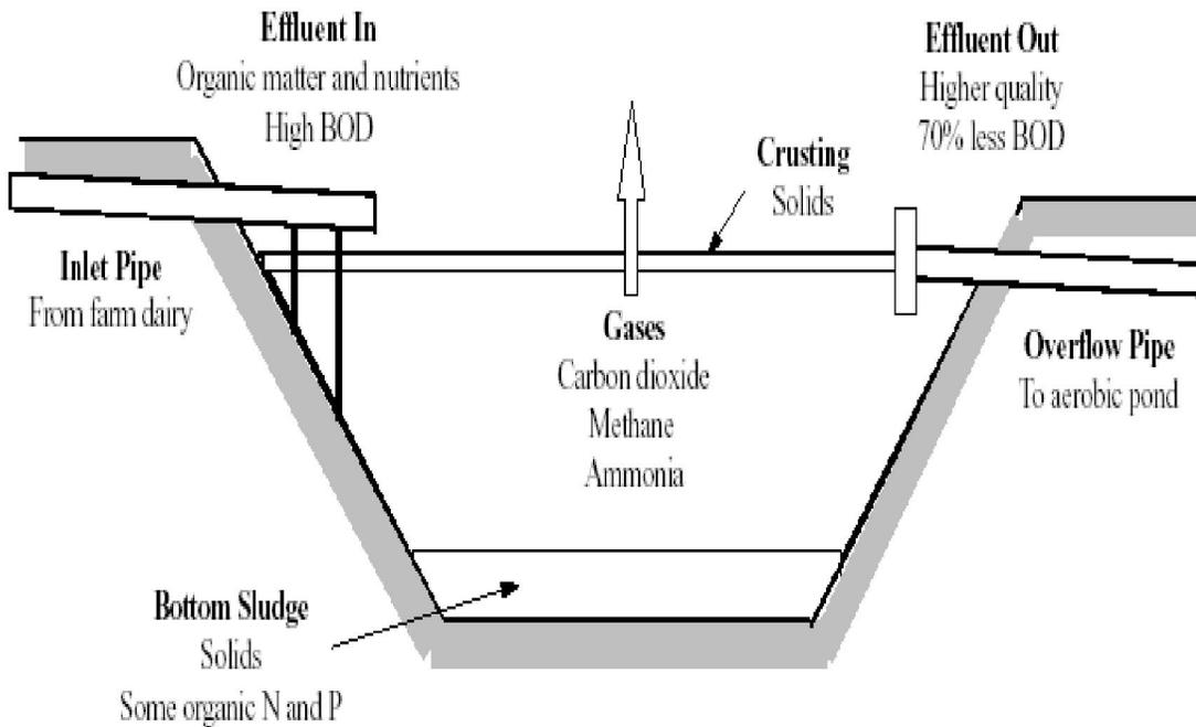
**Figure 2.2** Operation of the Anaerobic Pond.
