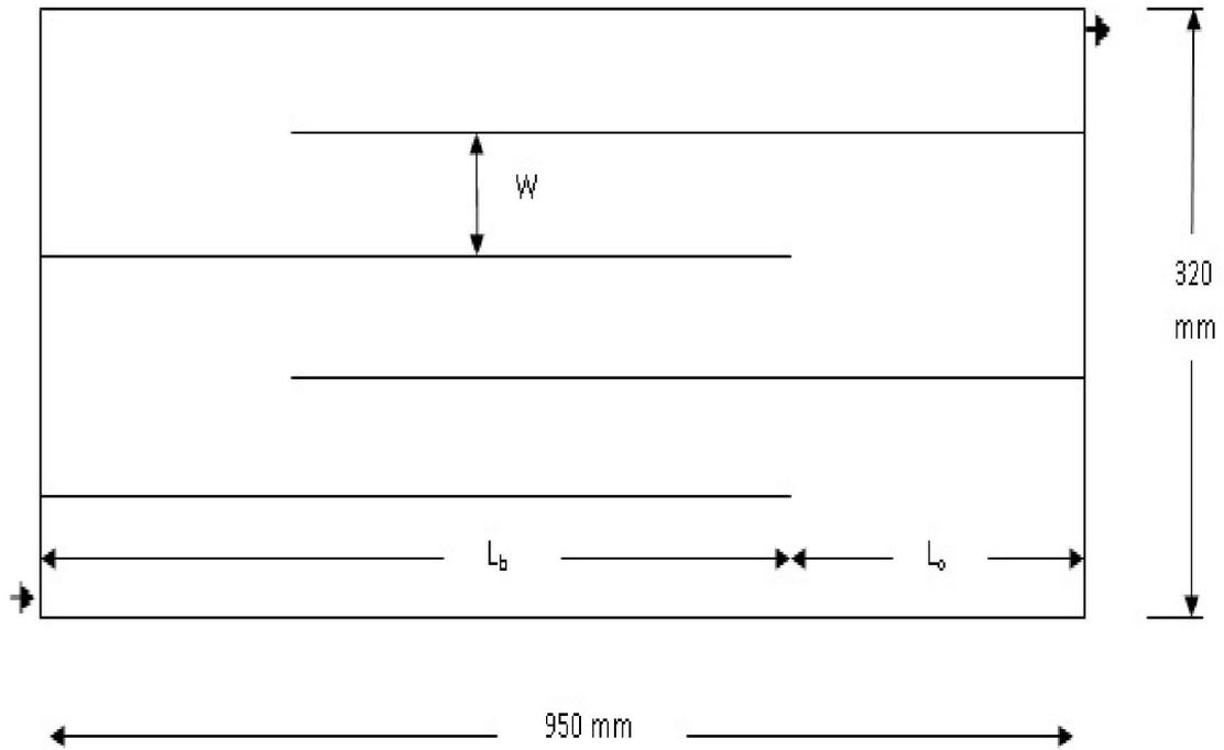
**Figure 3.15** General arrangements of conventional longitudinal baffles of different lengths in the anaerobic reactor
