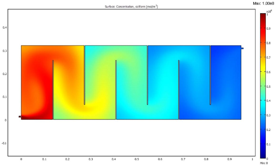
**Figure 4.33** Faecal coliform inactivation in a transverse 6-baffle 80% pond width anaerobic reactor
