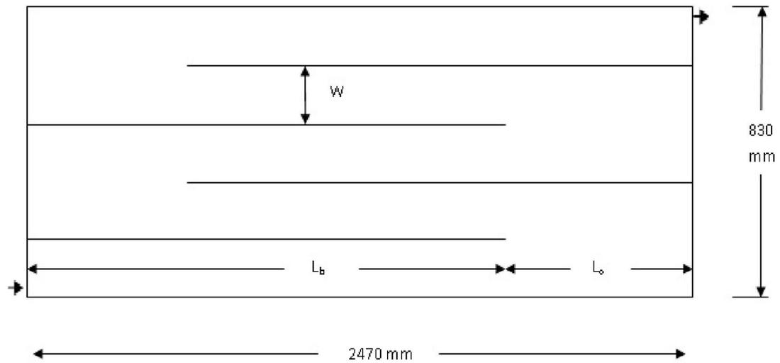
**Figure 3.17** General arrangements of conventional longitudinal baffles of different lengths in the maturation reactor.
