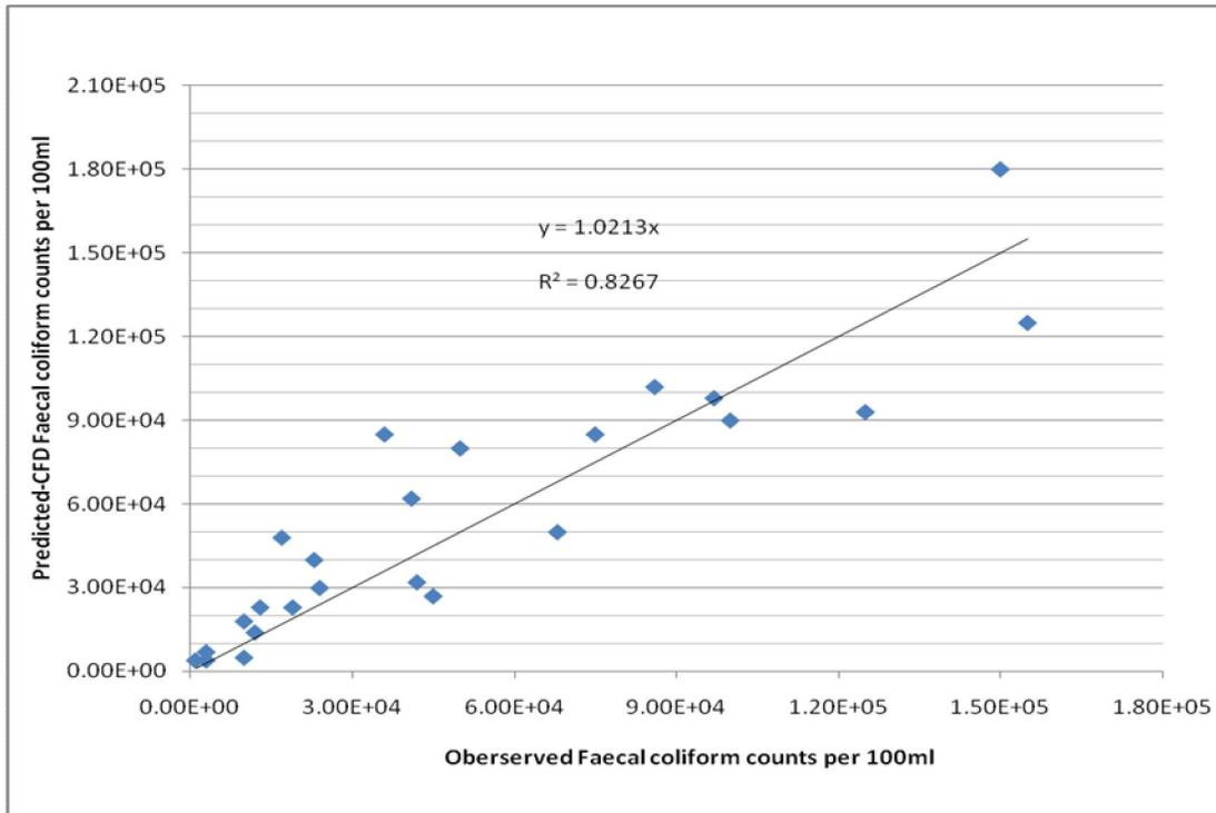
**Figure 3.14** Correlation data of the predicted-CFD and observed effluent Faecal coliform counts in baffled pilot-scale ponds. Source: Banda (2007).
