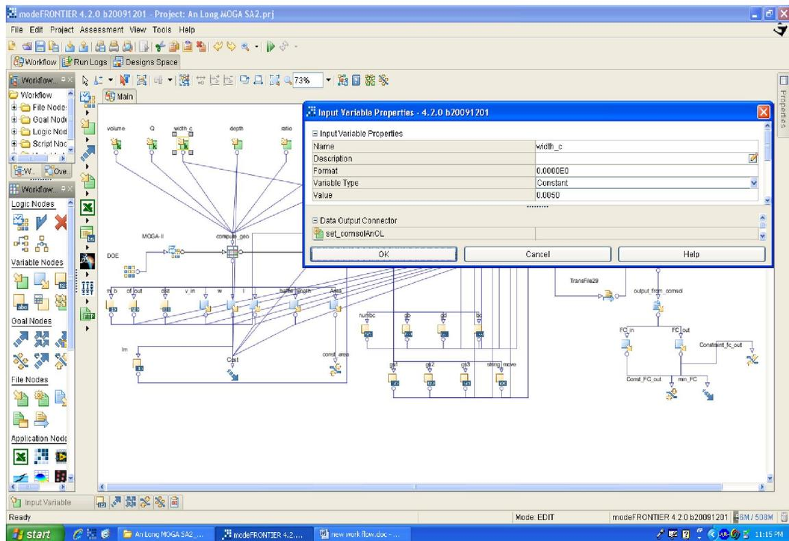
**Figure 3.26** Data variable carrying nodes and the input variable properties dialogue interface
