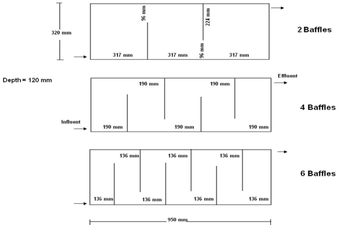
**Figure 3.5** Different baffle arrangements with 70% pond width anaerobic reactors
