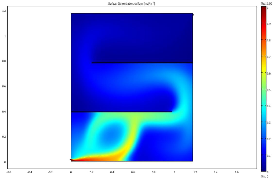
**Figure 4.46** SIMPLEX optimal faecal coliform removal design for combination of even and odd longitudinal baffle arrangement in facultative reactor
