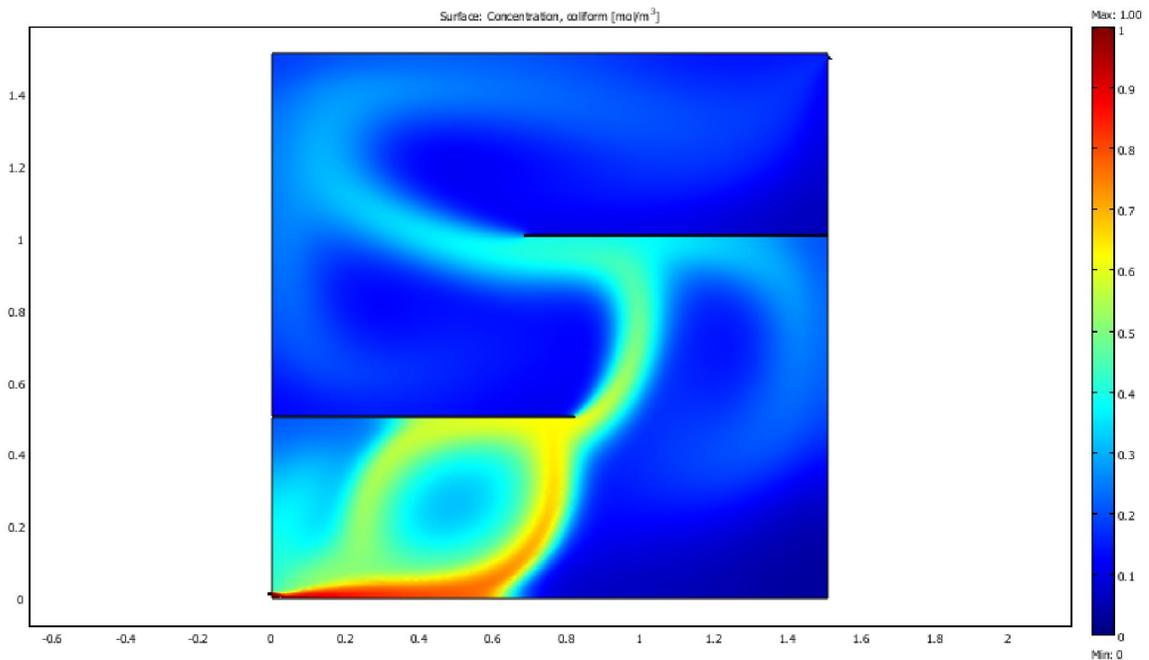
**Figure 4.89** MOGA II sensitivity analysis optimal faecal coliform removal design with least cost for longitudinal baffle arrangement in maturation reactor ( $k = 4.562$ )
