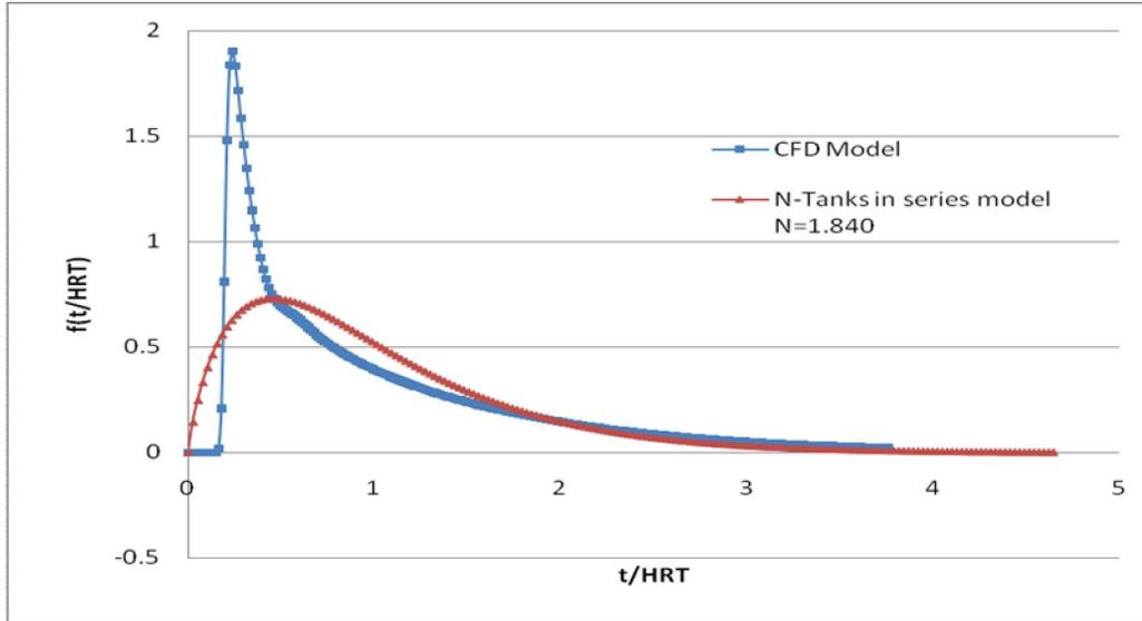
**Figure 4.29** Comparison of residence time density curves in 2-baffles, 80% pond width Maturation reactor for CFD and N-tanks in series models.
