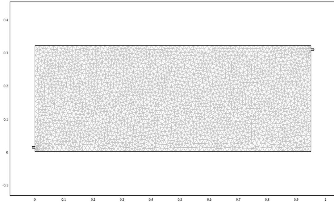
**Figure 3.10** Triangular meshes for the model anaerobic reactor
