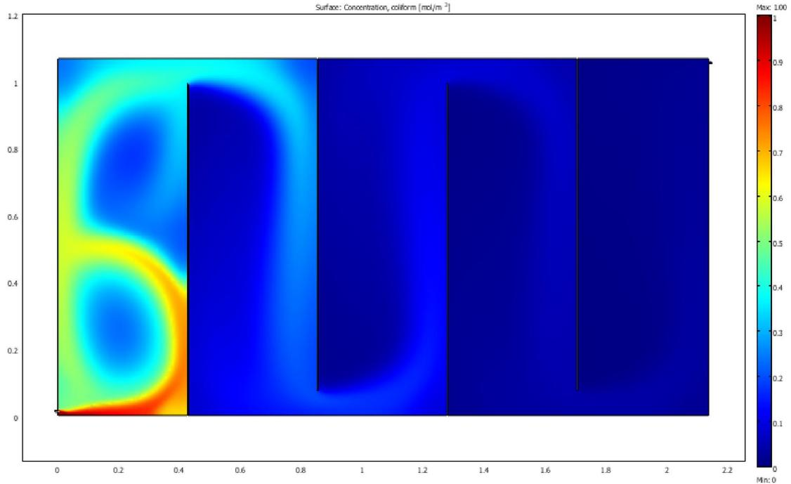
**Figure 4.57** MOGA-II optimal faecal coliform removal design with least cost for even baffle transverse arrangement in maturation reactor
