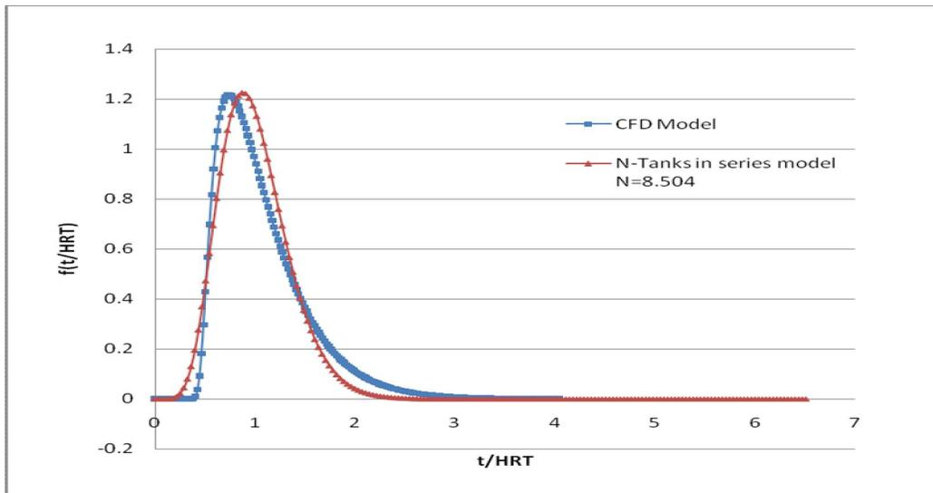
**Figure 4.28** Comparison of residence time density curves in 6-baffles, 80% pond width Facultative reactor for CFD and N-tanks in series models.
