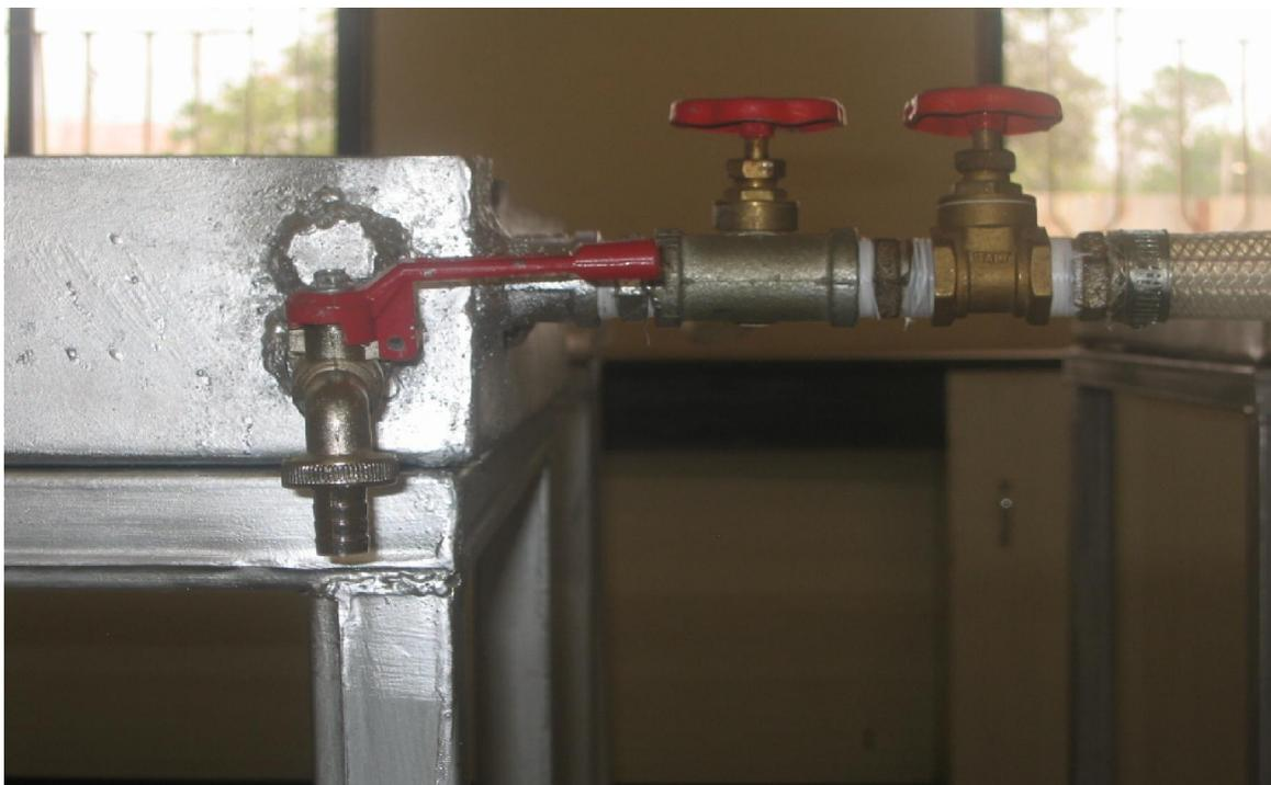
**Plate 3.13** Inlet and outlet structure of the laboratory-scale waste stabilization pond
