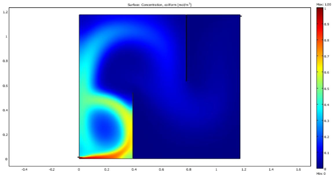
**Figure 4.79** MOGA II sensitivity analysis optimal faecal coliform removal design with least cost for transverse baffle arrangement in facultative reactor ( $k = 13.686$ )
