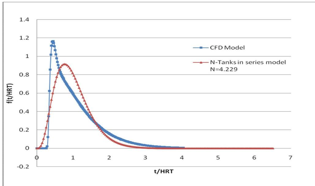
**Figure 4.21** Comparison of residence time density curves in 4-baffles, 70% pond width Facultative reactor for CFD and N-tanks in series models.
