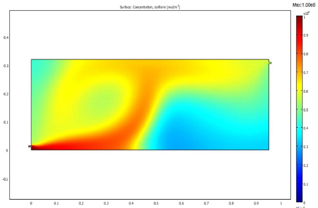
**Figure 4.2** Anaerobic un baffled reactor coliform inactivation
