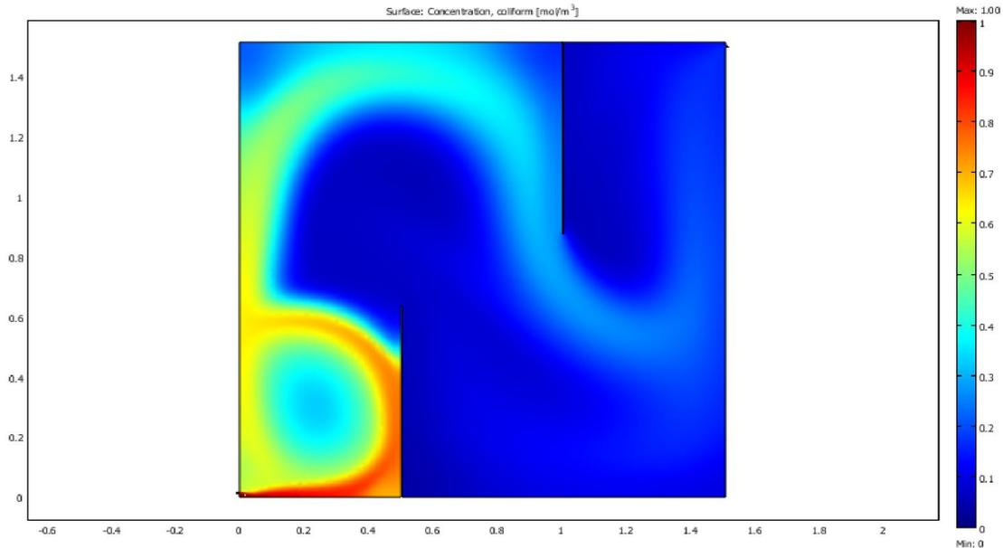
**Figure 4.86** MOGA II sensitivity analysis optimal faecal coliform removal design with least cost for transverse baffle arrangement in maturation reactor ( $k = 4.562$ )
