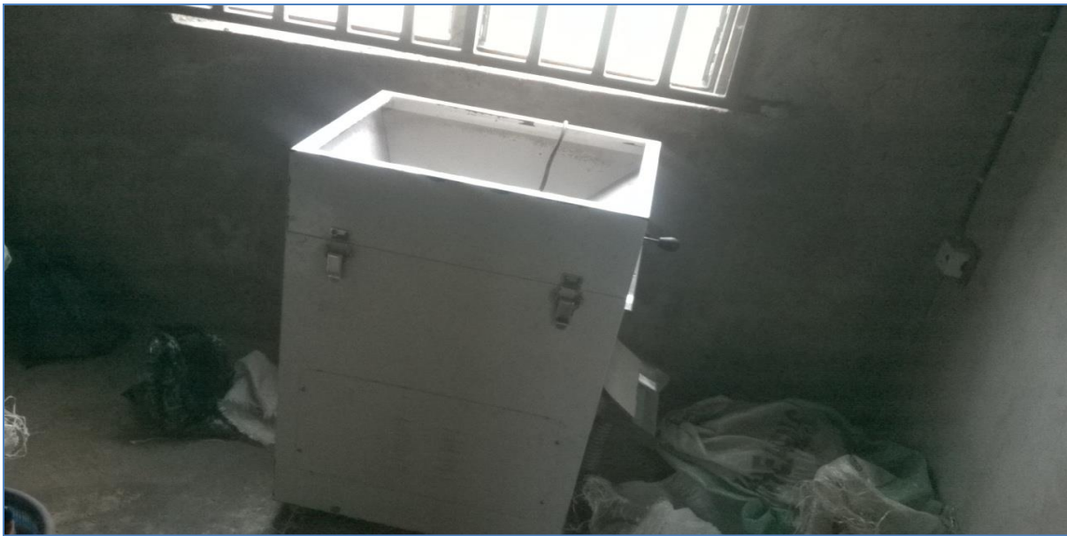
Figure A3: Stone Removal Machine ( Destoner ) Source: Fieldwork, 2016
