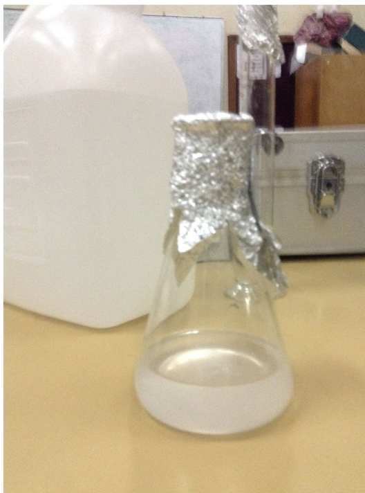
Figure 3. Image of the mixture of KOH and methanol.
