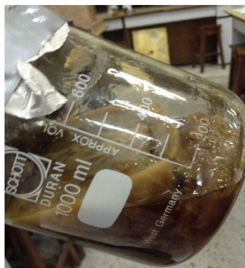
Figure 2. Incomplete production of biodiesel with WVO ethanol using KOH as catalyst.
