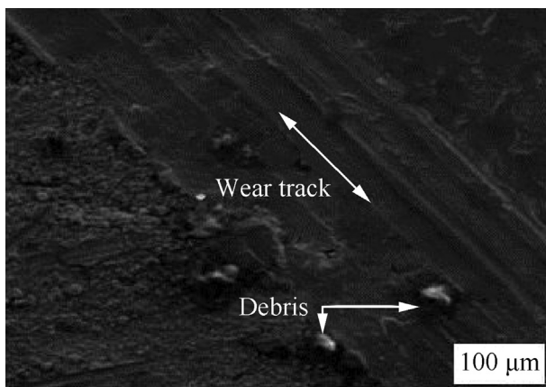
Fig. 14. SEM/EDS spectra showing the surface morphology of wear track (Zn-Al-7Sn-Ti-Cl-0.3 V deposition).
