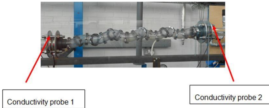
Fig. 2a Test section showing the PST and the conductivity rings
