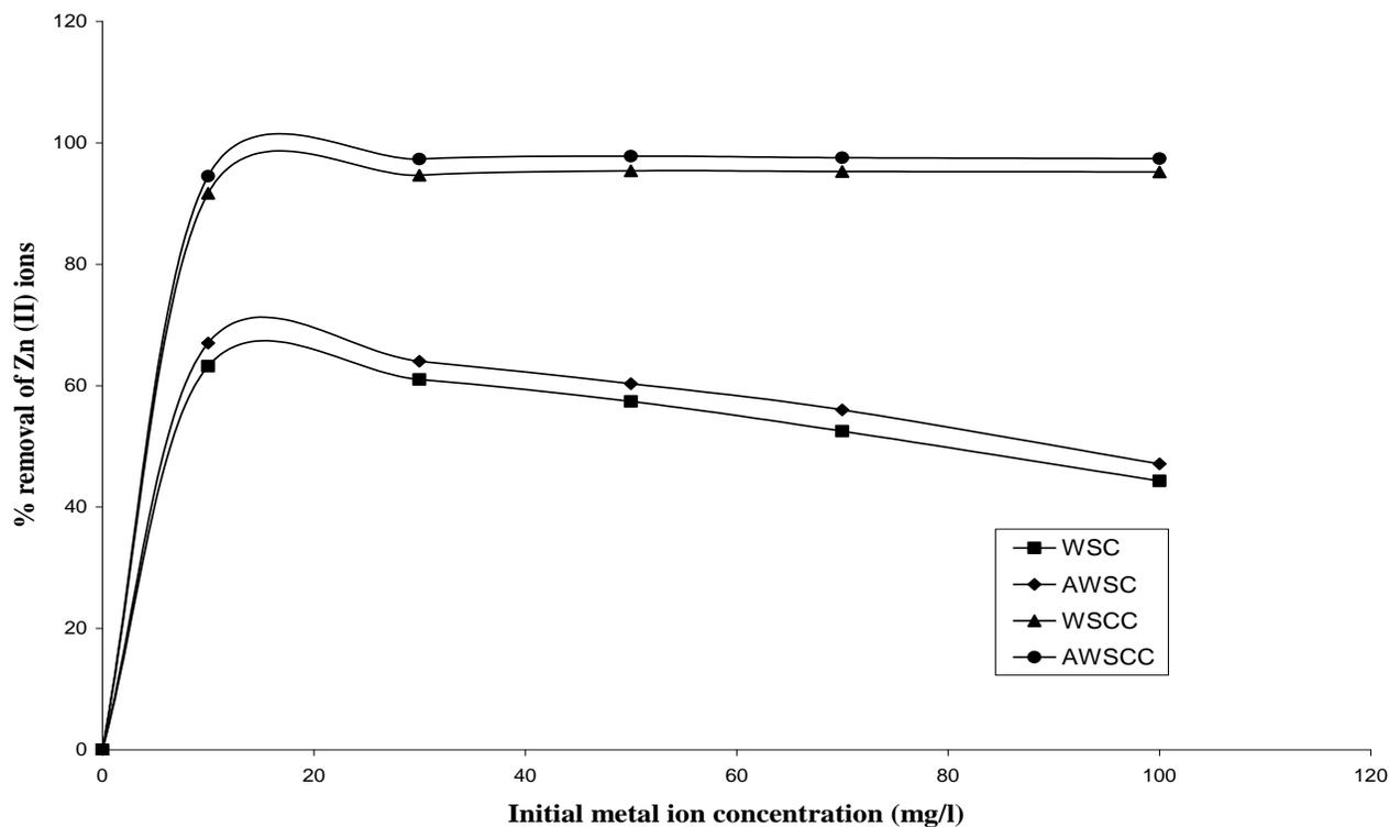
**Figure 3.** Effect of initial metal ion concentration on the removal efficiency of Zn (II) ions using WSC, AWSC, WSCC and AWSCC at pH=5, dose of each adsorbent=1 g, agitation speed=150 rpm, contact time=120 min, particle size=60BSS and temperature of solution=30°C.
