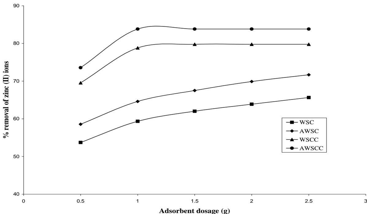
**Figure 2.** Effect of adsorbent dosage on the removal efficiency of Zn (II) ions using WSC, AWSC, WSCC and AWSCC at  $c_0 = 30$  mg/L, pH=5, agitation speed=150 rpm, contact time=120 min, particle size=60BSS and temperature of solution=30°C.
