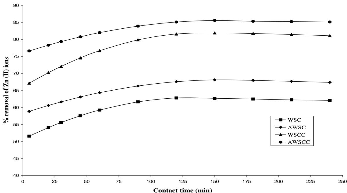
**Figure 4.** Effect of contact time on the removal efficiency of Zn (II) ions using WSC, AWSC, WSCC and AWSCC at  $c_0 = 50$  mg/L, pH=5, dose of each adsorbent=1 g, agitation speed=150 rpm, contact time=120 min, particle size=60BSS and temperature of solution=30°C.
