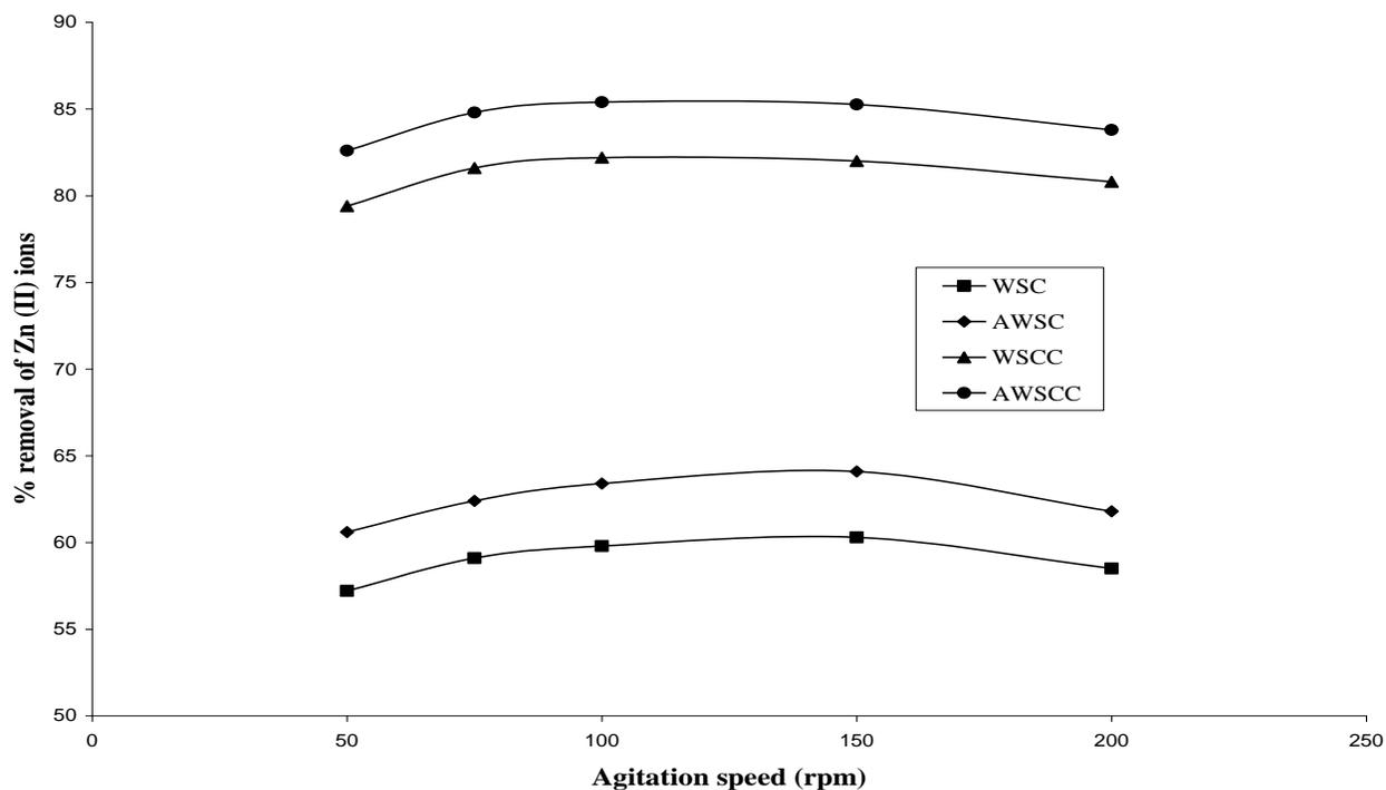
**Figure 5.** Effect of agitation speed on the removal efficiency of Zn (II) ions using WSC, AWSC, WSCC and AWSCC at  $c_0 = 50$  mg/L, dose of each adsorbent=1g, agitation speed=150 rpm, contact time=120 min, particle size=60BSS and temperature of solution=30°C.
