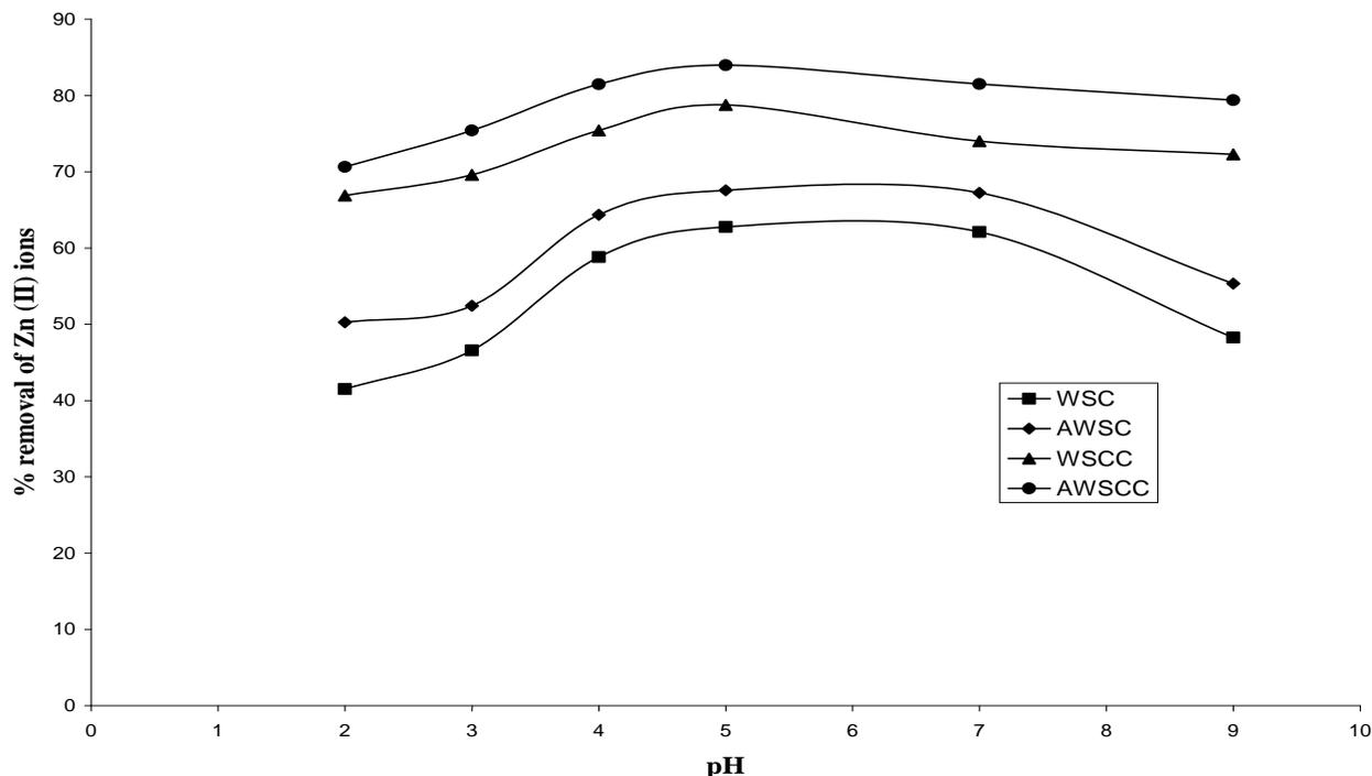
**Figure 1.** Effect of pH on the removal efficiency of Zn (II) ions using WSC, AWSC, WSCC and AWSCC at  $c_0 = 30$  mg/L, dose of each adsorbent=1g, agitation speed=150 rpm, contact time=120 min, particle size=60BSS and temperature of solution=30°C.
