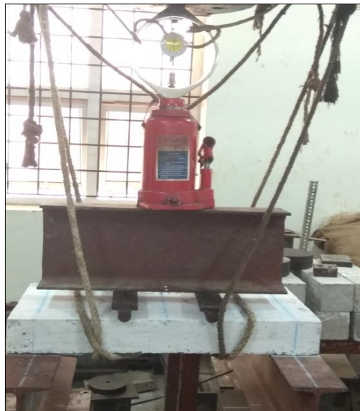
Fig. 3. Slab panel subjected to flexural strength test.
