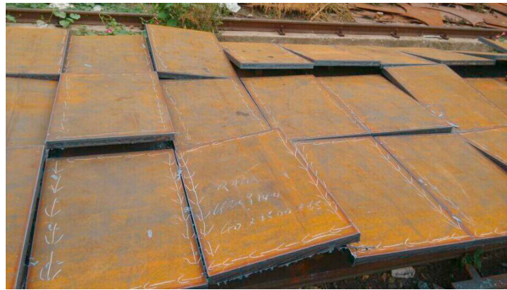
Figure 1: Atmospheric corrosion that is initiated by atmospheric particles
