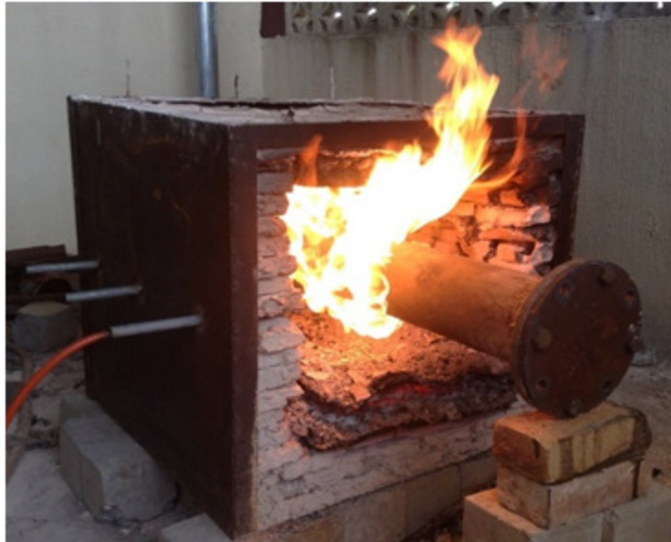
Figure 6 Test- Running the model Pyrolysis furnace[11].
