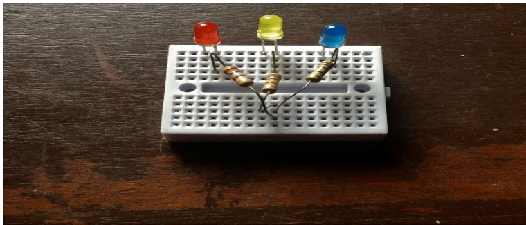
Figure 5: LEDs and resistor connection on the breadboard
