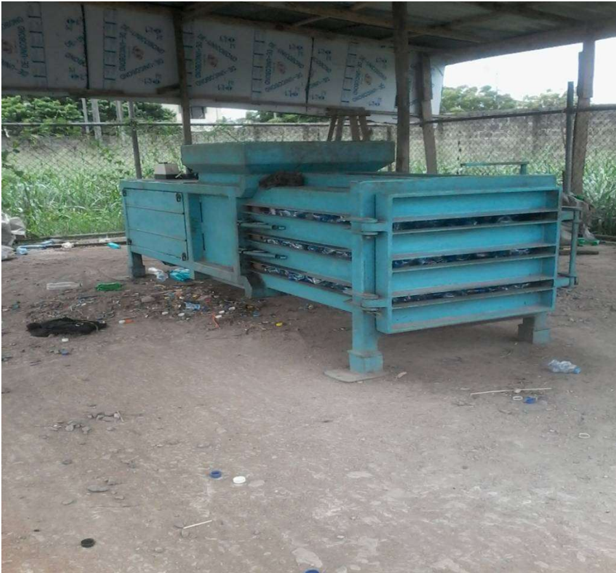
Baling machine used at WTW site
