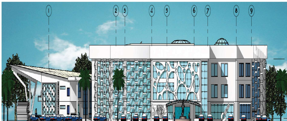
Figure 9: Elevation showing the anti-solar glass façade
