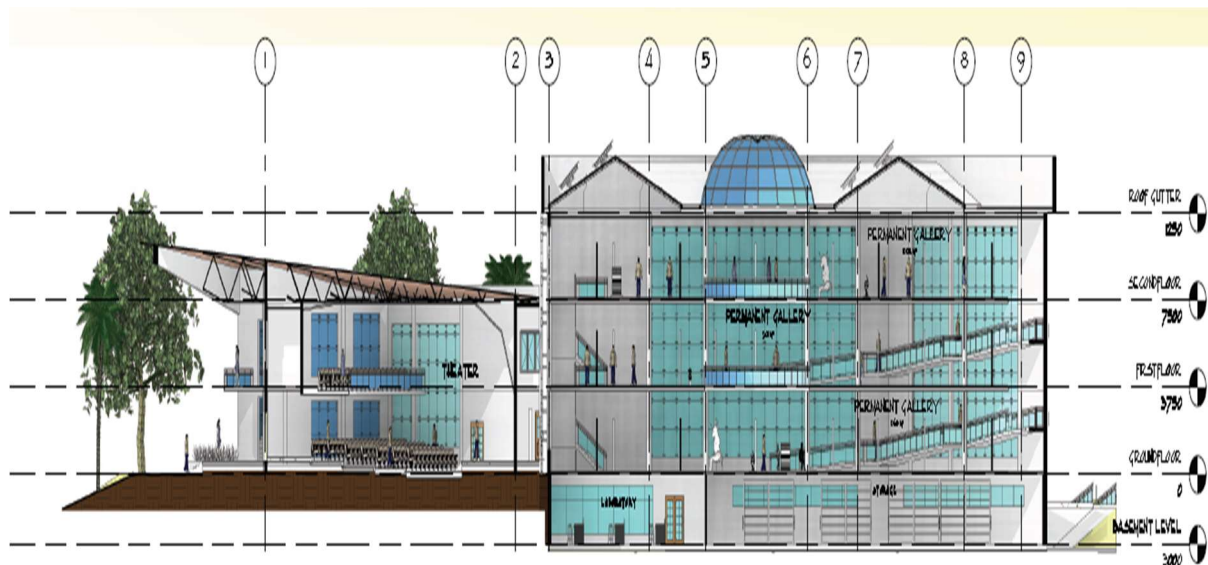
Figure 8: Section BB showing the photovoltaic installation and the overhang cantilever
