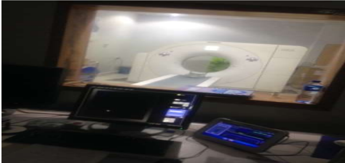
Plate 1: Computed tomography room through the lead glass used to protect the operator's area.
