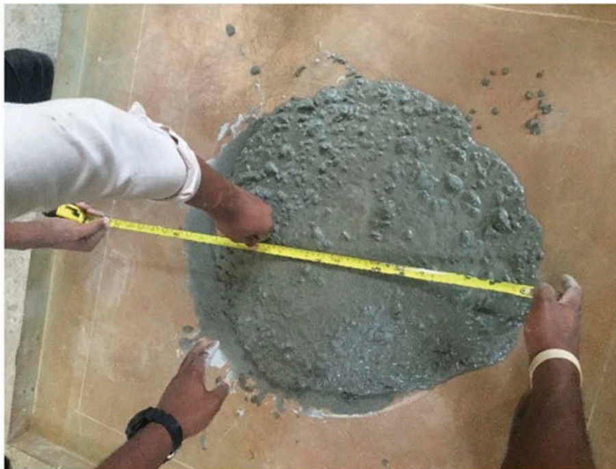
Figure 6. (a) Slump flow test; (b) V-funnel test.
