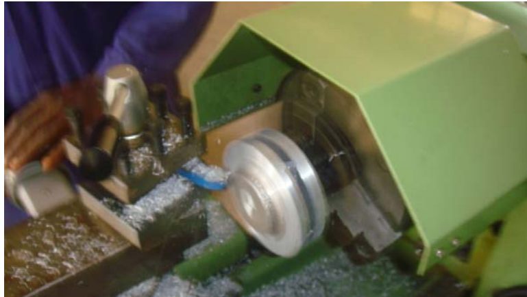
Figure 1: Impeller undergoing machining operation on the lathe machine
