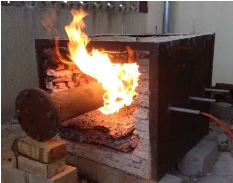
Figure 6: Test- Running the model Pyrolysis furnace
