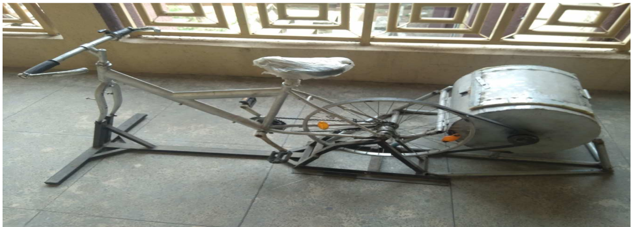
Figure 7. Complete Assembly of the Human powered pedal washing machine.
