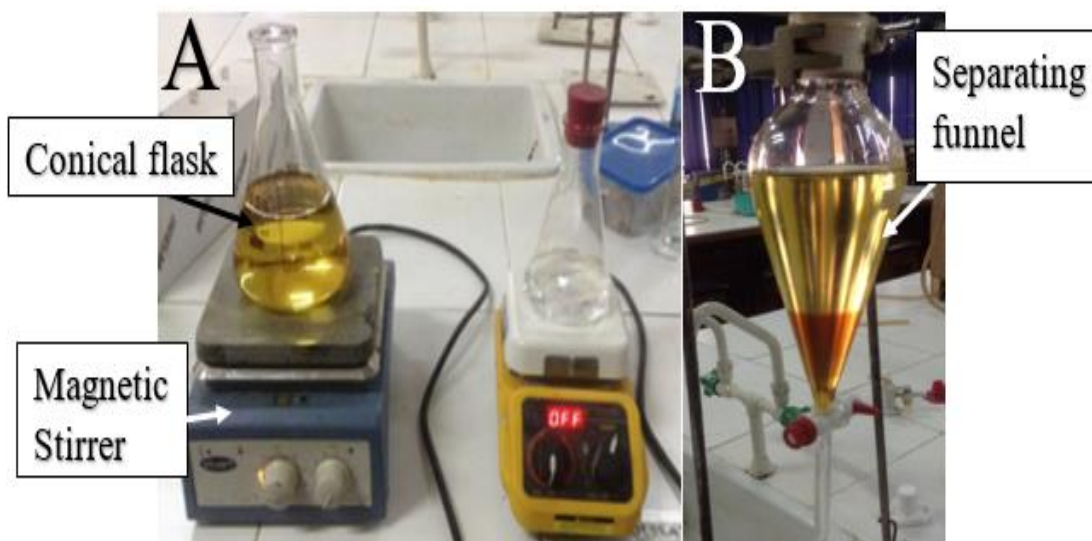
Figure 1: (A)-Oil Heating in Conical Flask and Mixture of Methanol and KOH. (B)- Separation of Product into Crude Biodiesel and Glycerol
