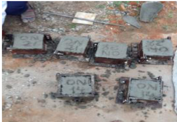
Fig. 3. Casting of concrete cubes.
