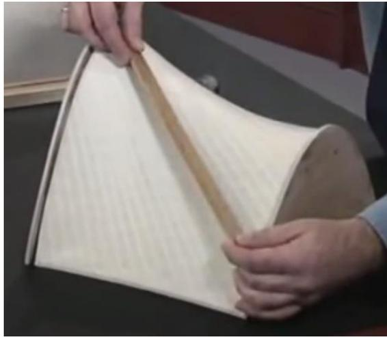
Plate 3. 12: Ruler laid flat on the surface of hyperbolic paraboloid
