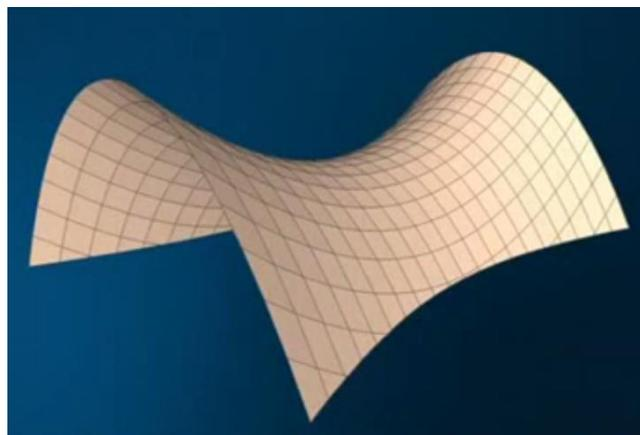
Plate 3. 5: Saddle forms have double curvature in opposite directions
