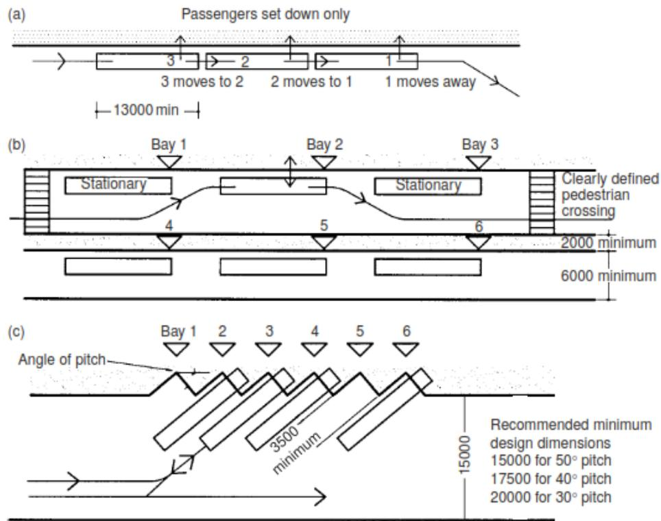
Figure 2. 11: The way buses approach platforms a) shunting, b) drive-through c) sawtooth
