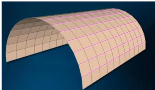
Plate 3. 3: Cylinders have curvature in one direction only
