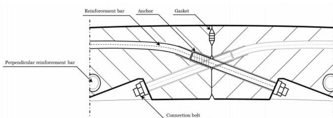
Figure 3. 8: Detailed connection between thin-shell prefab elements using bolted connection
