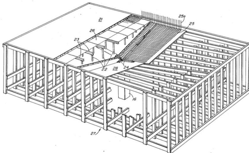
Figure 3. 4: Perspective partial cutaway view of several layers of forms and reinforcement materials usable in hyper umbrella
