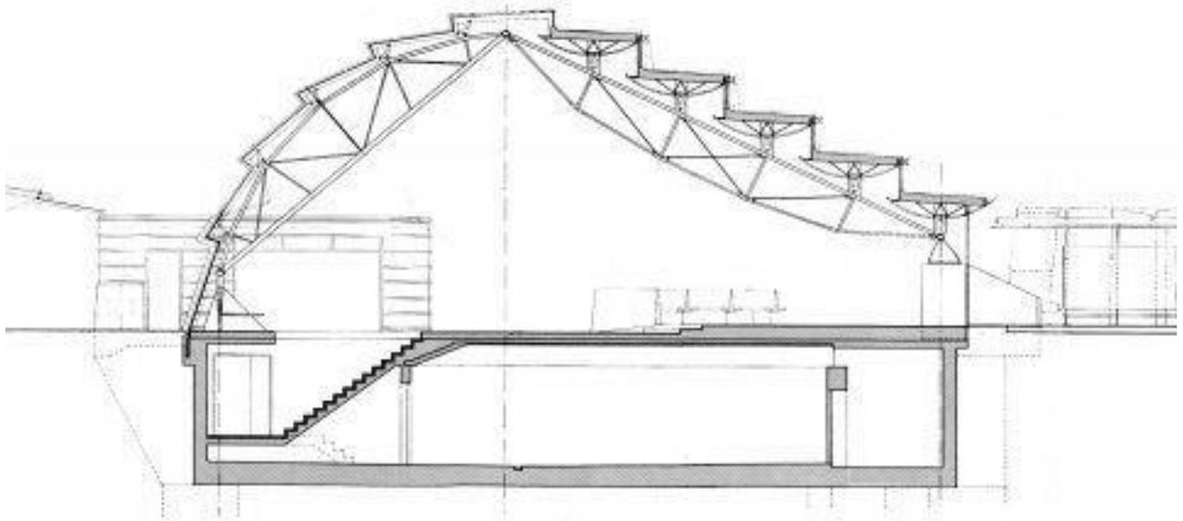
Figure 4. 3: Section of the Nil Ericson terminal, showing the large hall and the basement garage
