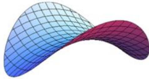
Plate 3. 10: The pringle chip is another example of a double curvature surface
