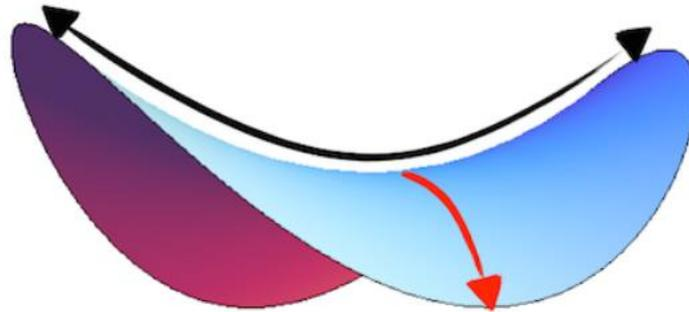
Plate 3. 14: The red arrow represents compression and the black arrow represent tension
