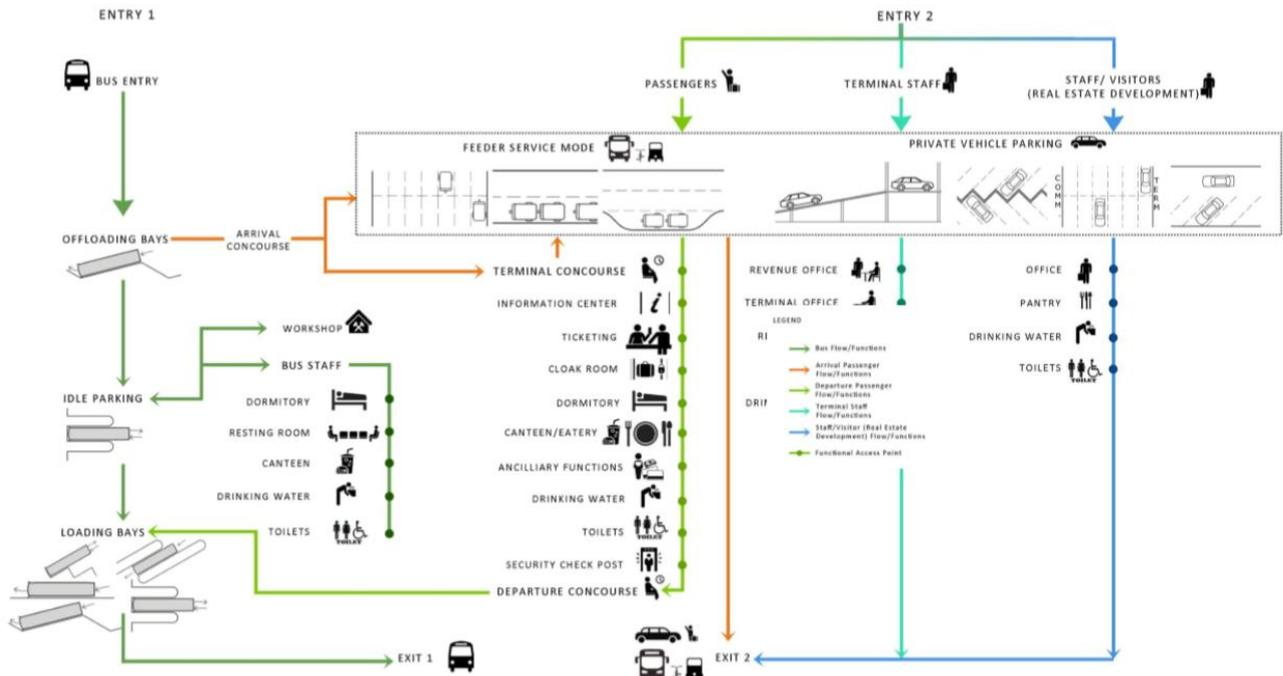
Figure 7. 10: Bus terminal passenger flow chart
