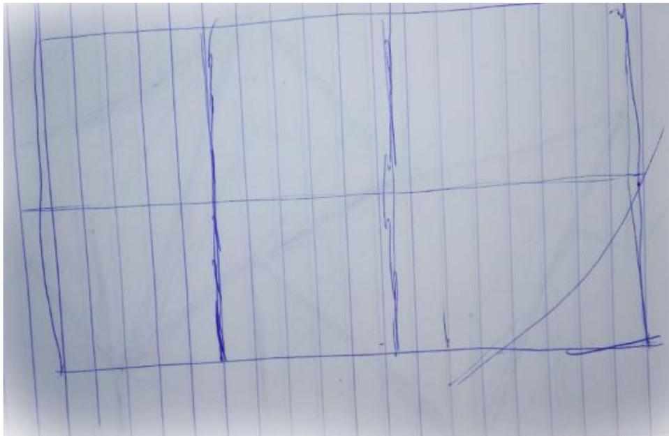
Plate 7. 4: Initial hand sketch of the roof structure divided into three bays
