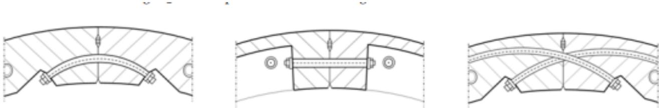
Figure 3. 10: Connection location between thin-shell concrete elements
