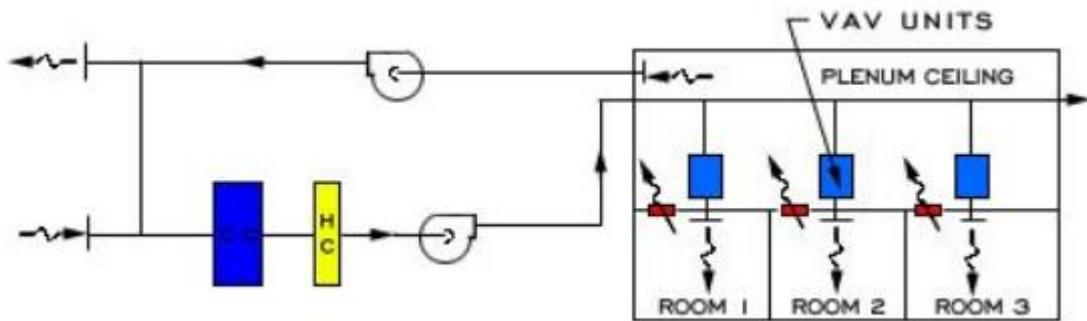
Figure 2. 13: All-Air central system diagram of the category variable air volume (VAV)
