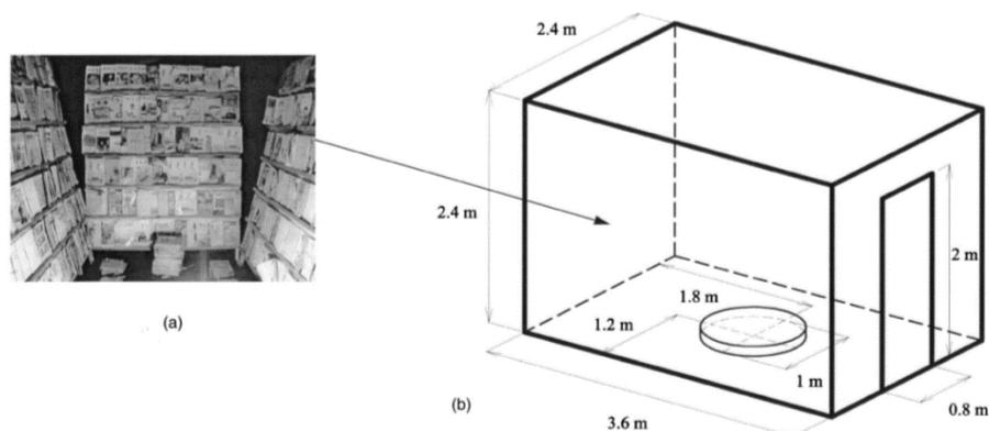
Figure 2. 15: This is the newspaper shop and its geometry where the fire test was performed.
