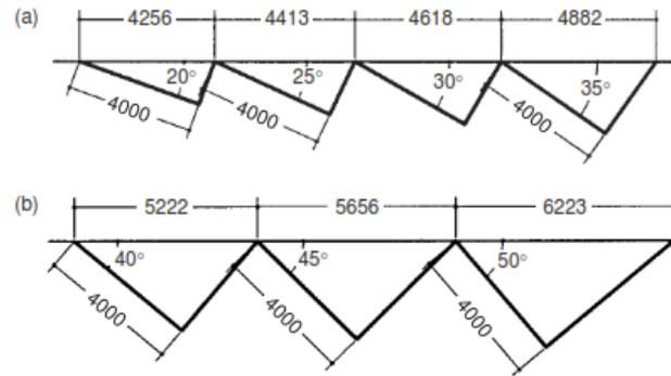
Figure 2. 12: Dimension and angles in sawtooth configuration
