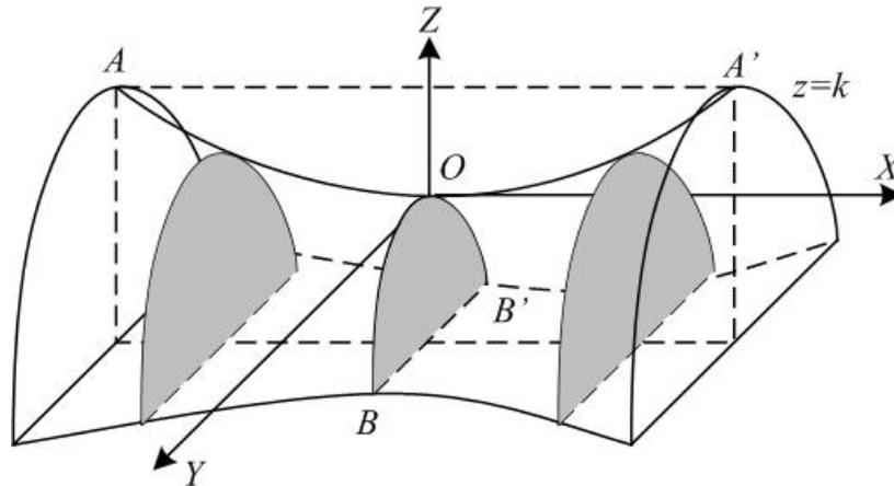
Plate 3. 6: Parabolic curve shaped extruded along a hyperbolic curve
