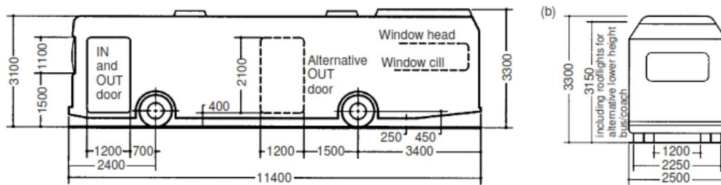
Figure 2. 7: Typical length and width of a bus
