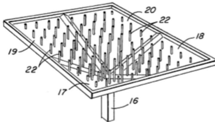
Figure 3. 6: Perspective view of the hyper of umbrella without the slab
