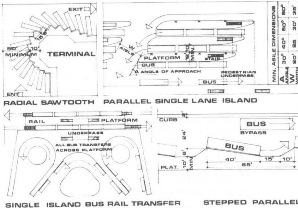
Figure 2. 10: Types of bus loading platform
