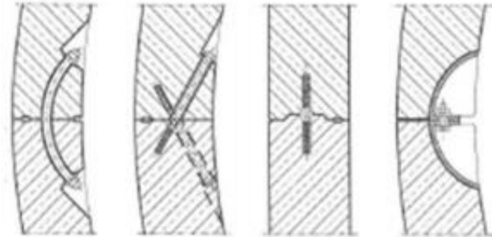
Figure 3. 7: Bolt connection joint in concrete
