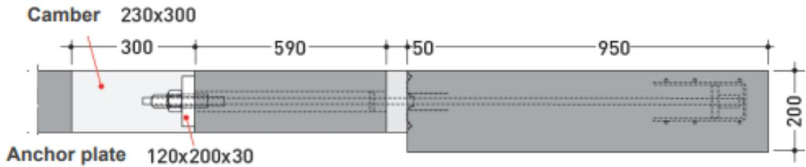
Figure 3. 9: Section of fixation of precast element to existing structure using post-tension connection
