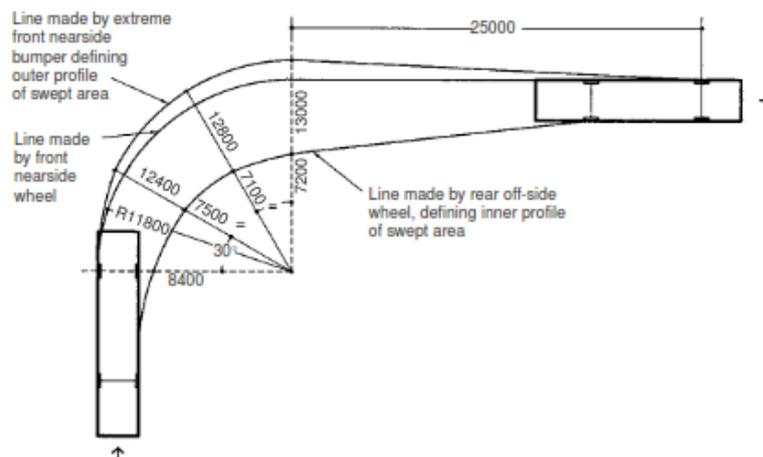
Figure 2. 8: Shows a 10 m bus making a turn of 90 degrees
