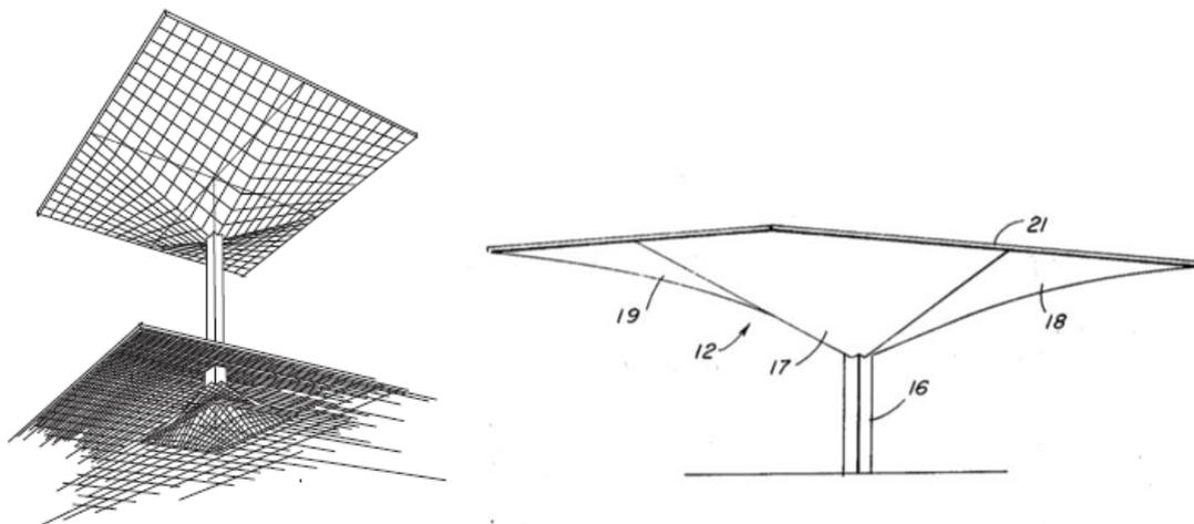
Figure 3. 2: On the left is the hyper umbrella on its foundation and on the right is its frontal view
