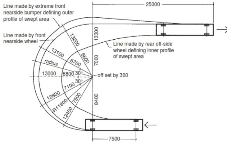
Figure 2. 9: A bus of length 12 m making a turn of 180 degrees
