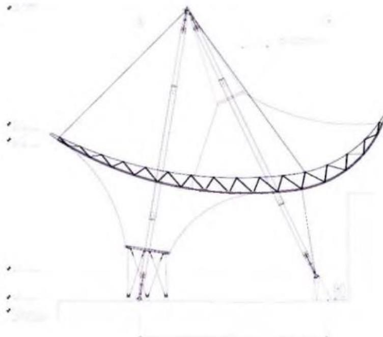
Figure 4. 8: Section showing the canopy structure
