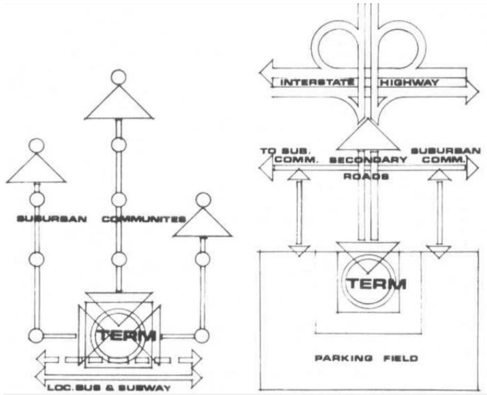
Figure 2. 4: On the lefthand side is urban-suburban commuter terminal, on the righthand side is suburban
