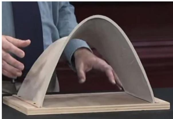
Plate 3. 11: View of the parabolic shape on the hyperbolic paraboloid
