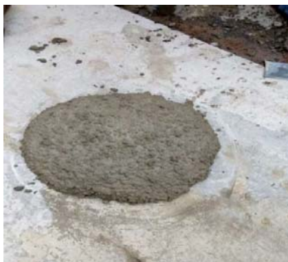
Figure 2. Slump flow test
