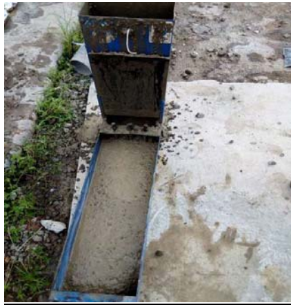
Figure 4. showing the L-box test
