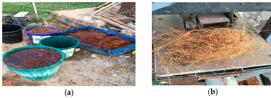
Figure 1. (a) Coconut fibres soaked in water. (b) Coconut fibres after being extracted from the husk.
