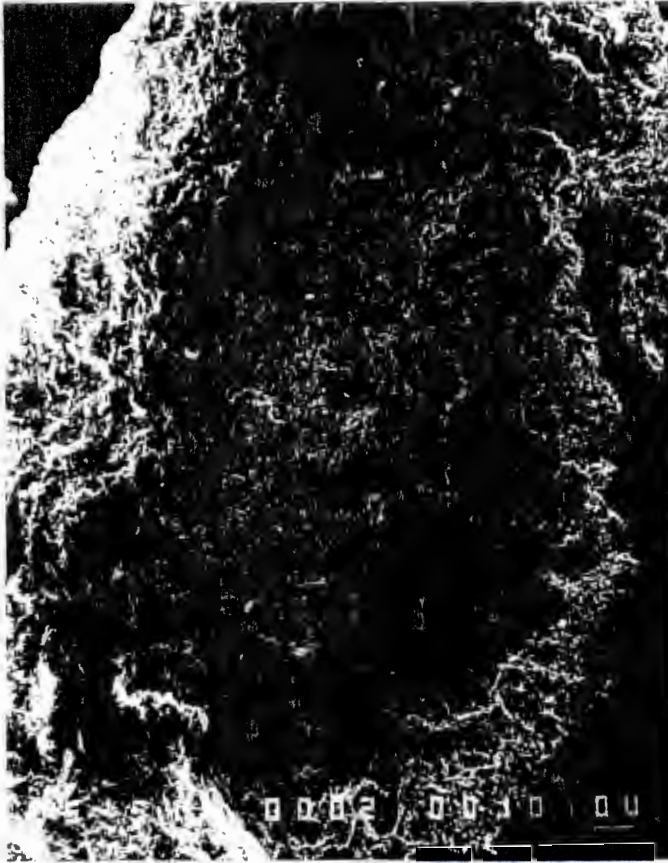
Fig. 2. SEM micrograph of Igbokoda clay particle showing the surface structure and the particle shape ( \times 1000 ).
