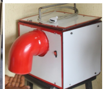
A Non-contact Solar/Electric powered Automated Soap-Water Dispenser and a high speed Non-contact Electronic Sanitizer Dispenser produced by Prof Omoleye's Research Team in 2020
