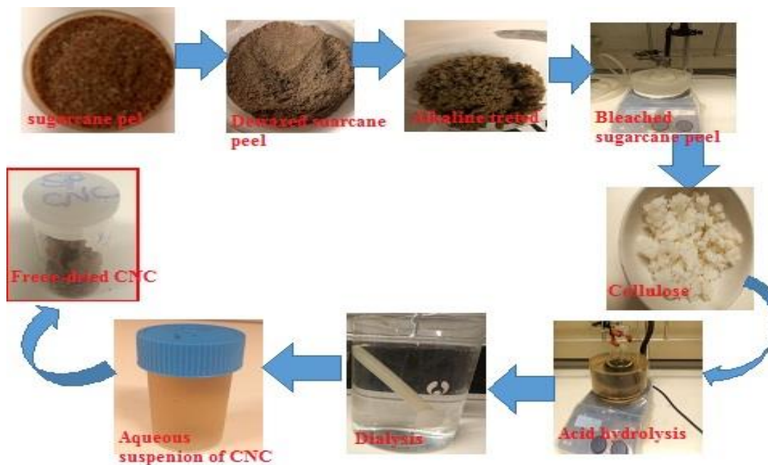
Fig. 1. Schematic representation of the preparation of cellulose nanocrystals from sugarcane peel
