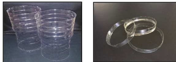
Fig. 6. Ring-shaped plastic fibres used for improved concrete beam performance [24].
