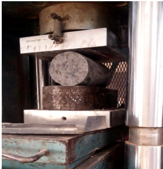
Fig. 2. Split Tensile Strength Test.
