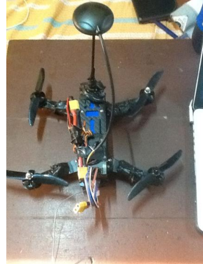
Fig 2. The Assembled Quadcopter (As built)
