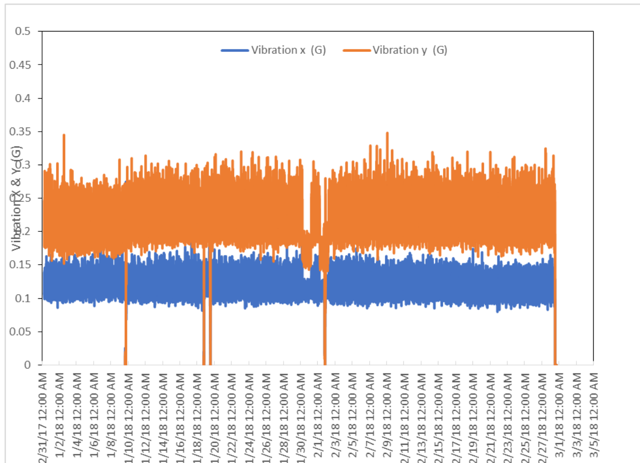
Figure 3. Vibration Data Chart for Oil Field Operating ESP
