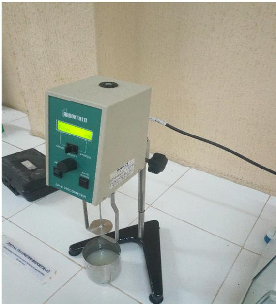
Fig. 8. Measurement with Brookfield DV-E Viscometer.
