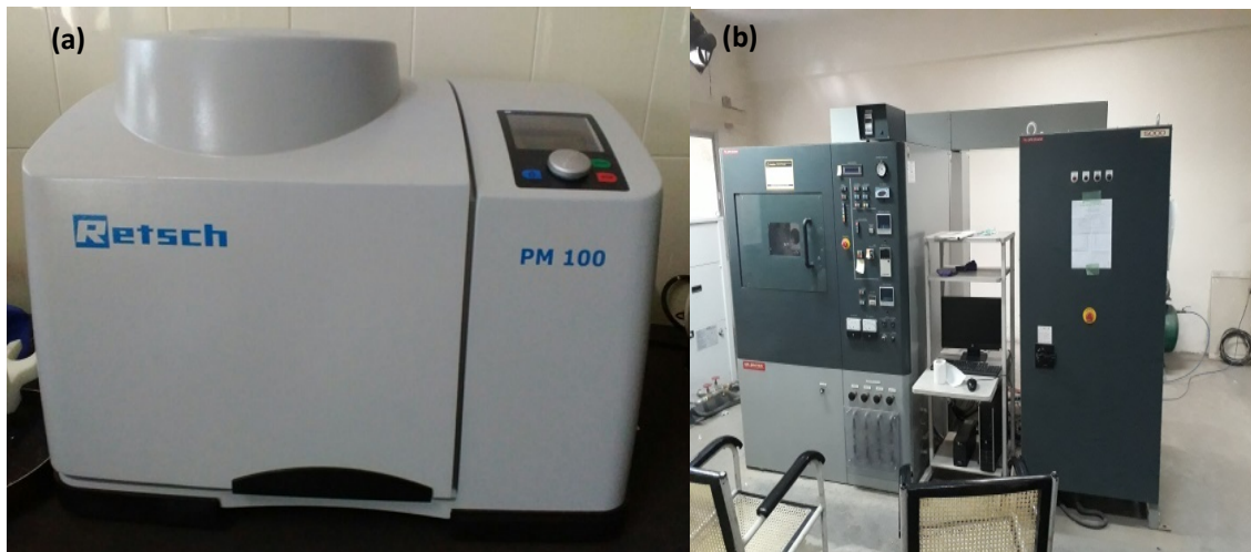
Figure 2: (a) High energy planetary ball mill, (b) Spark plasma sintering (SPS) machine
