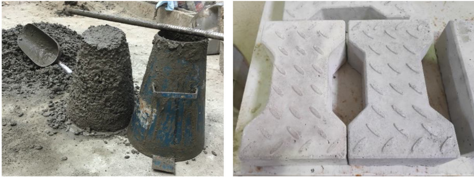
Fig. 5. Slump of concrete mix (left); Interlocking concrete paver block (right).
