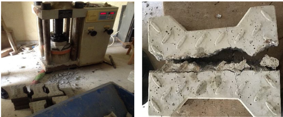
Fig. 6. Testing of interlocking concrete paver (left); Failure mode of the paver sample containing WSF (right).
