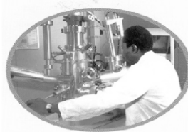
Examining top atomic monolayers of a material by Auger spectroscopy
