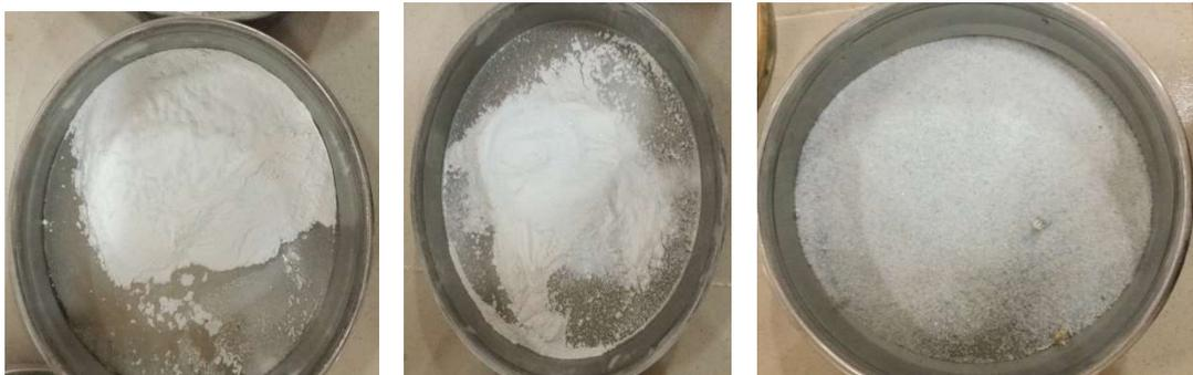
**Figure 1.** The waste glass particle sizes used: (a) <75  $\mu\text{m}$ , (b) <150  $\mu\text{m}$  but >75  $\mu\text{m}$ , and (c) <300  $\mu\text{m}$  but >150  $\mu\text{m}$
