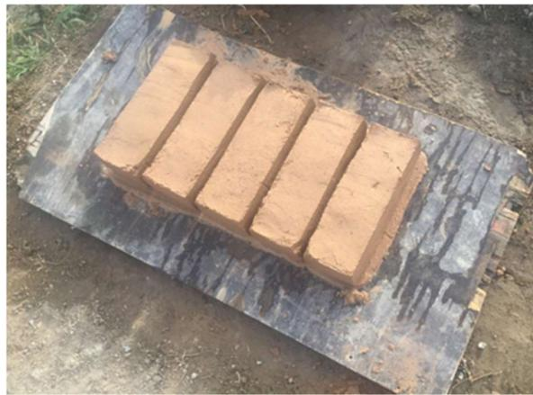
**Figure 2.** Some of the dried bricks before being fired in the furnace
