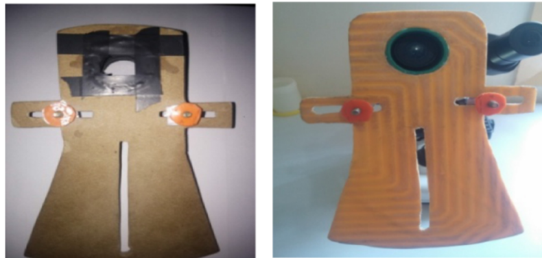
Fig. 2. The adapter prototype from wooden and plastic materials.
