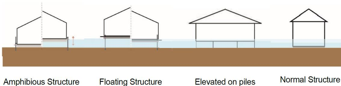
Figure 4.28: Types of Building Structures and their Action during Flooding
