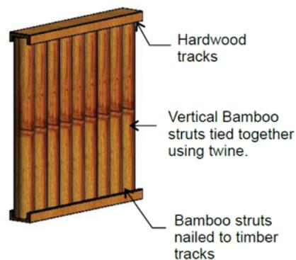
Figure 4.25: Walling Components made with Bamboo Sticks
