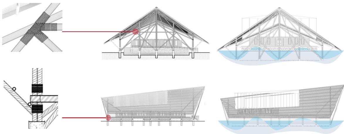
Figure 4.9: Platform Design Schematic Diagram
