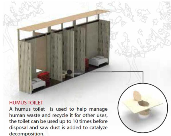
Figure 4.31: Humus Toilet Positioned in a Structure
