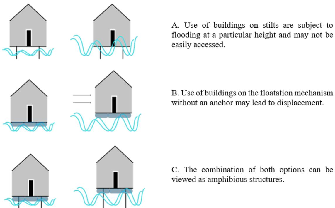
Figure 2.3: Principle of Amphibious Structure
