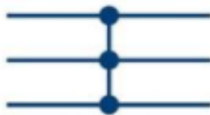
Figure 3 Three Phase short circuit fault
