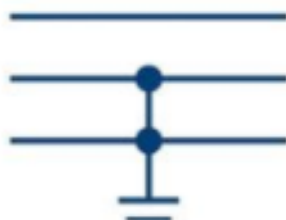
Figure 5 Double Line-to-Ground short circuit fault
