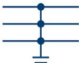
Figure 2 Three Phase-to-Ground fault
