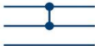
Figure 4 Line-to-Line short circuit fault
