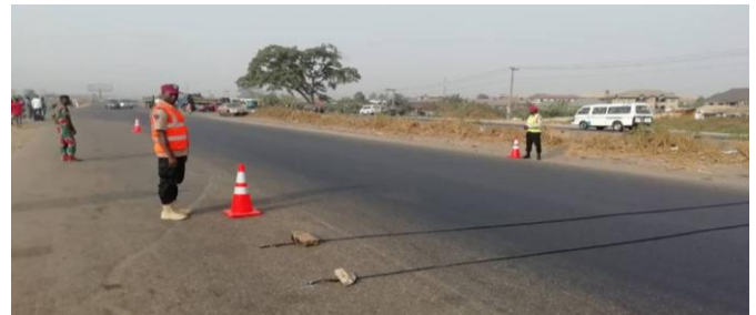
Figure 1: FRSC personnel using the MetroCount pneumatic road tube counter to record traffic count along the Lagos-Ibadan expressway (Federal Road Safety Corps, 2019)
